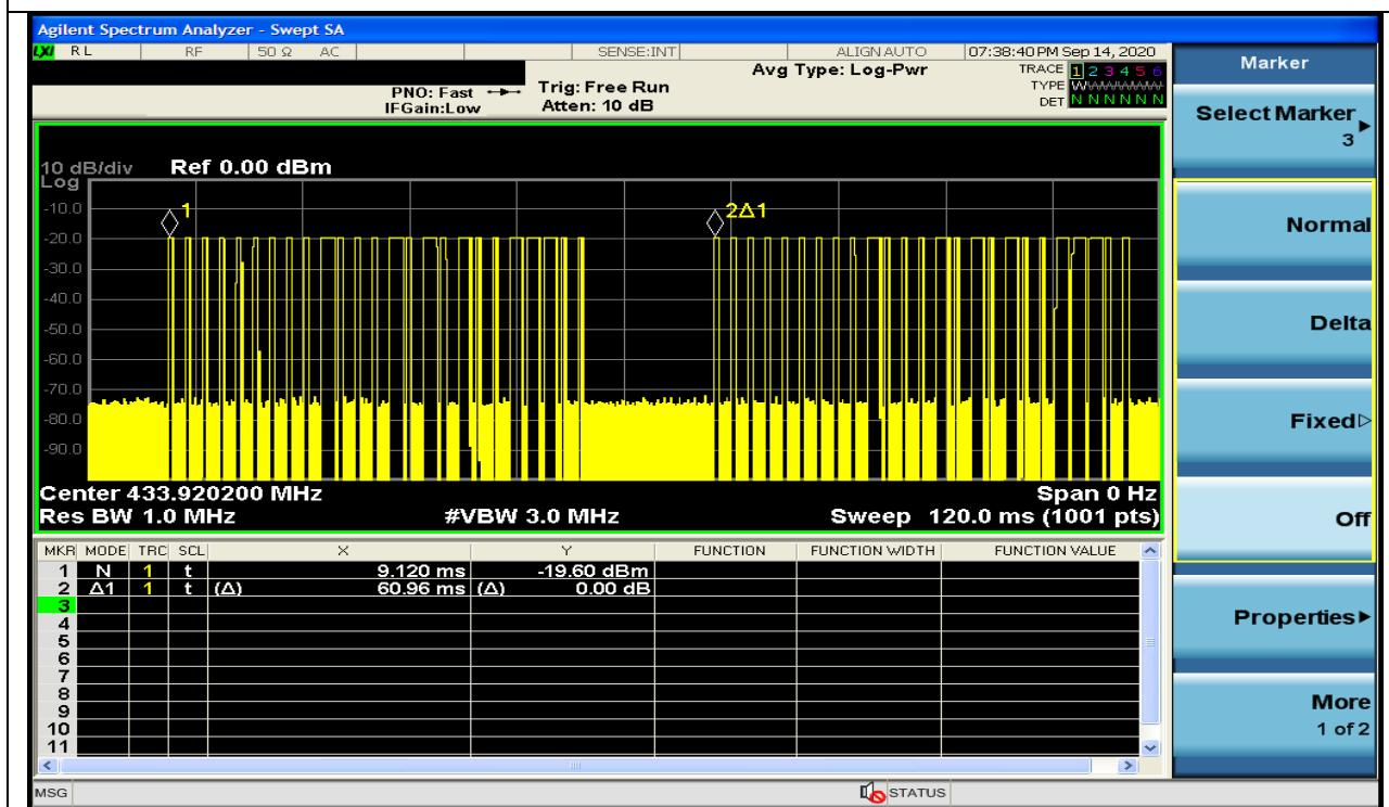
TX on=0.48\*18+1.44\*7=18.72ms, TX off=Tp-Ton=60.96-18.72=42.248ms
