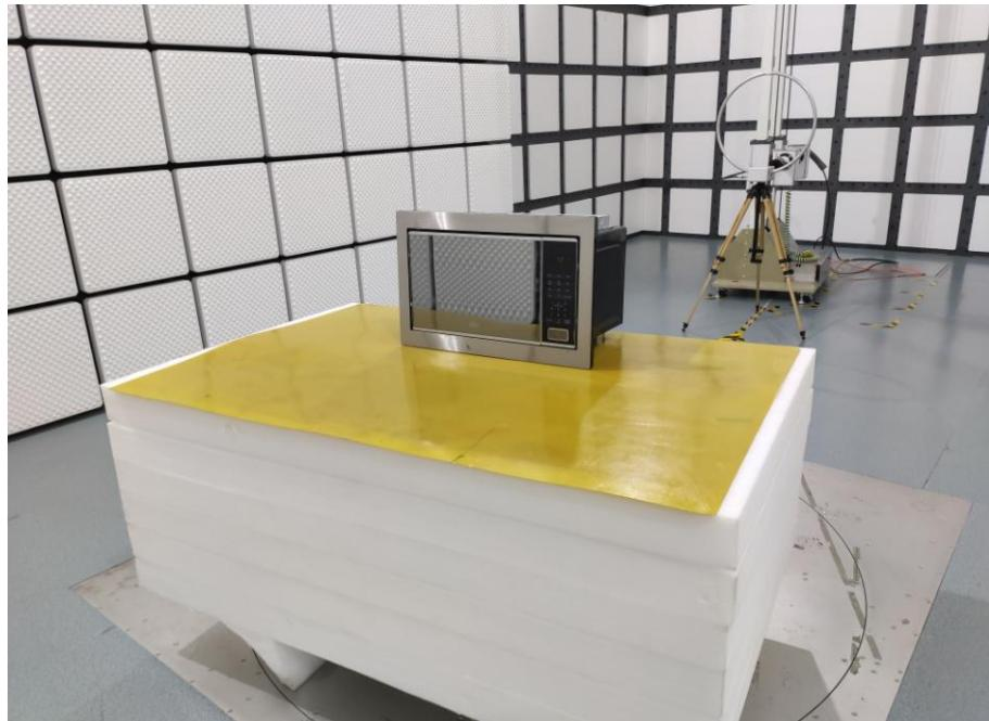
**Radiated Spurious Emissions Test View (30MHz-1GHz)**
