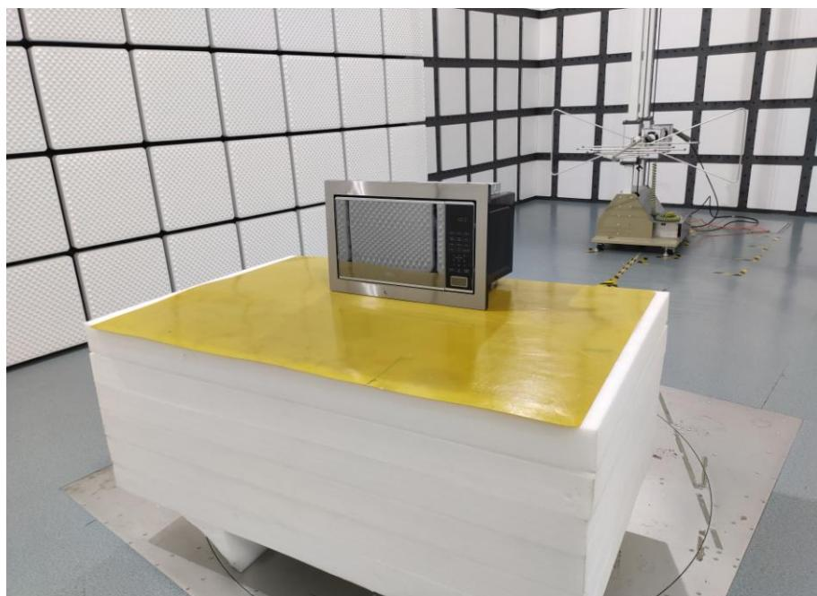
**Radiated Spurious Emissions Test View (Above 1GHz)**
