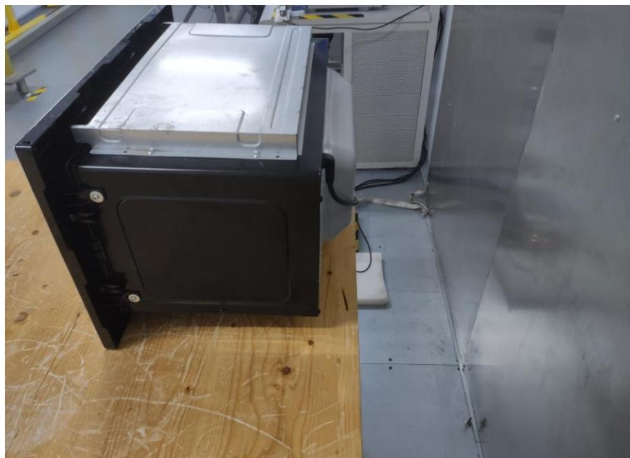
**Radiated Spurious Emissions Test View (Below 30MHz)**
