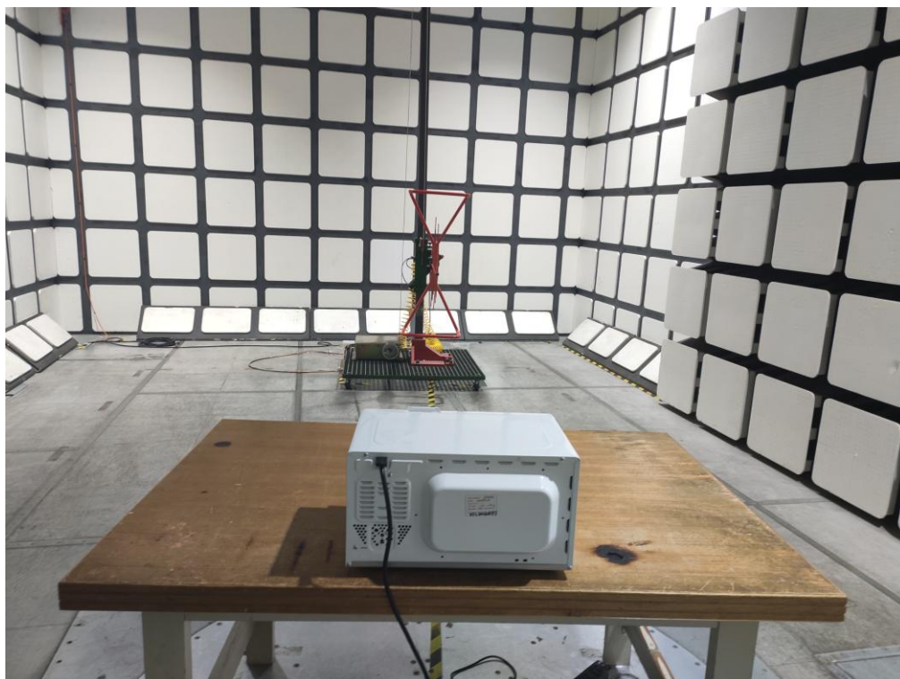
Radiated Emissions - Rear View (30 MHz – 1 GHz)
