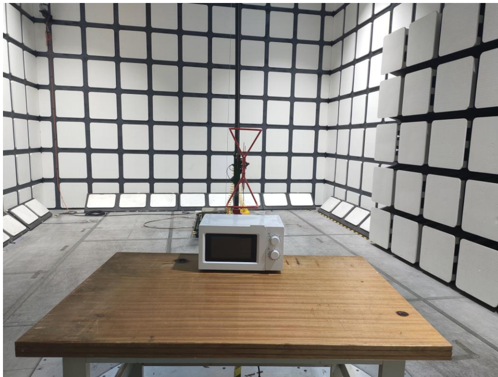
Radiated Emissions - Rear View (30 MHz – 1 GHz)
