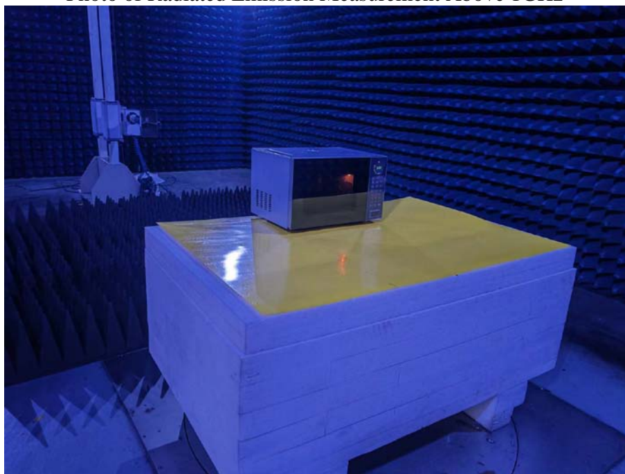
Photo of Radiated Emission Measurement Above 1GHz
