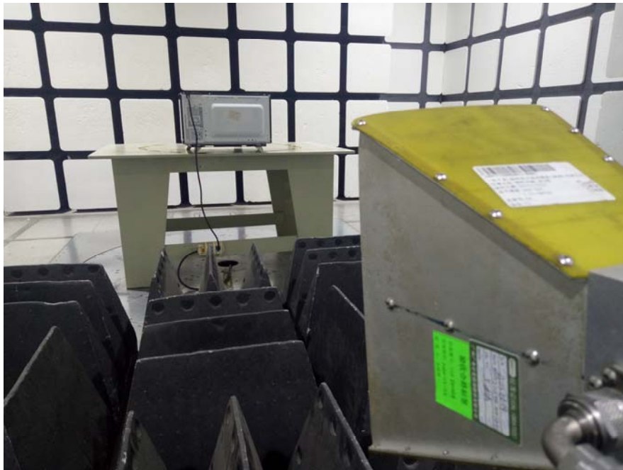
Radiated Emissions - Rear View (Above 1 GHz)
