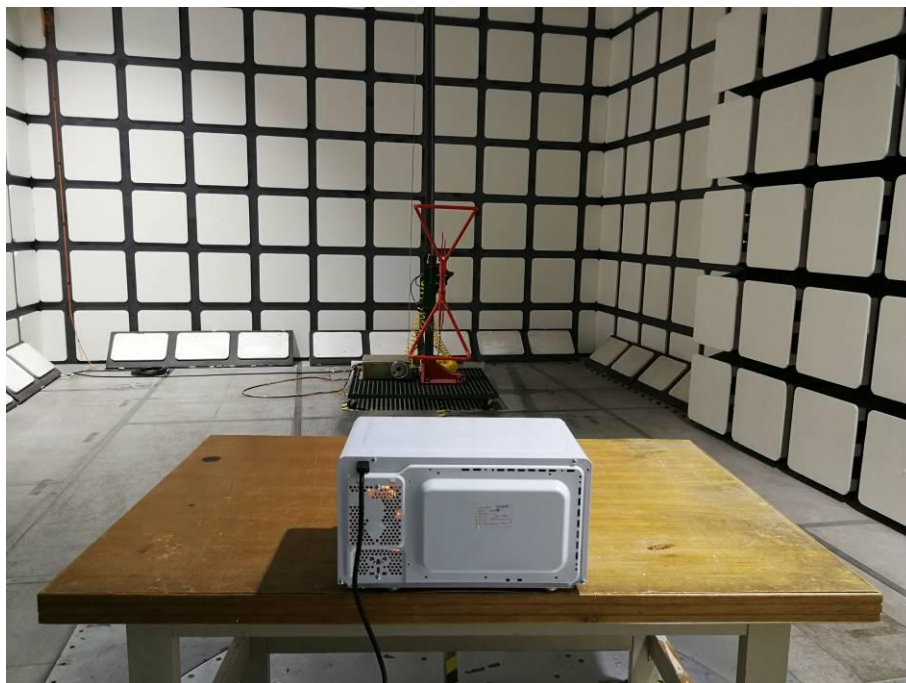
Radiated Emissions - Rear View (30 MHz – 1 GHz)
