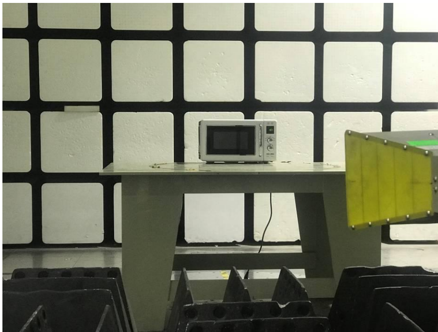
Radiated Emissions - Front View (Above 1 GHz)
