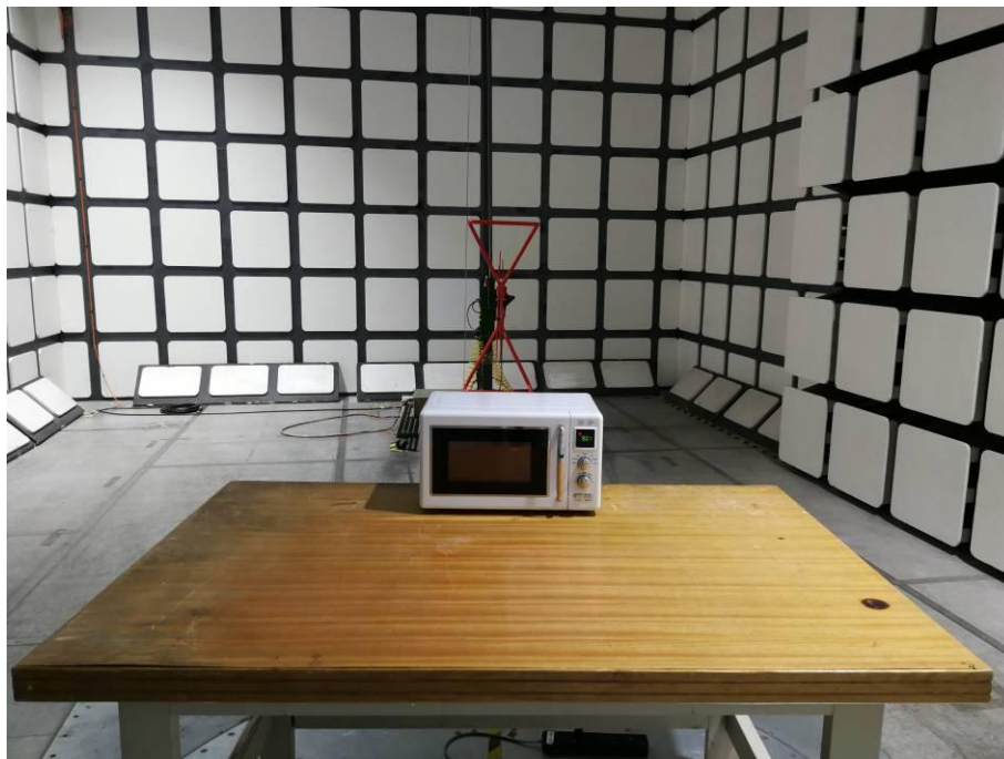
Radiated Emissions - Front View (30 MHz – 1 GHz)
