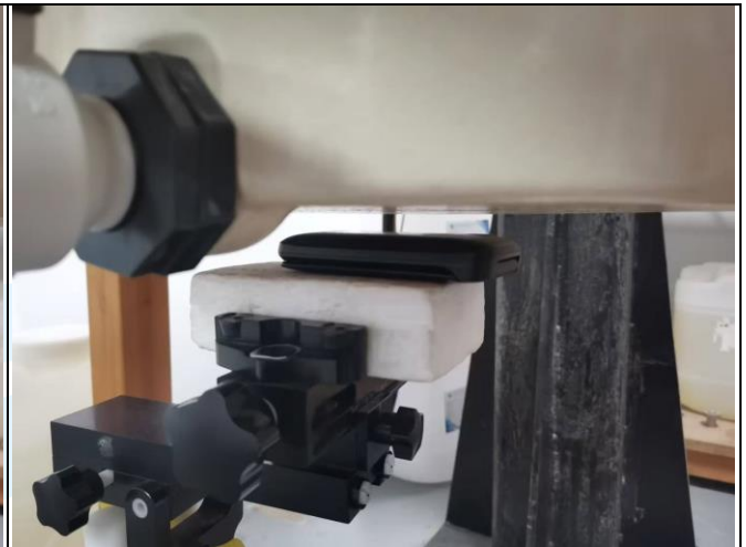
Rear Face of EUT with 1.0 cm Gap
