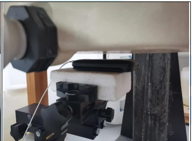
Rear Face of EUT with 1.0 cm Gap (ERPHONE)
