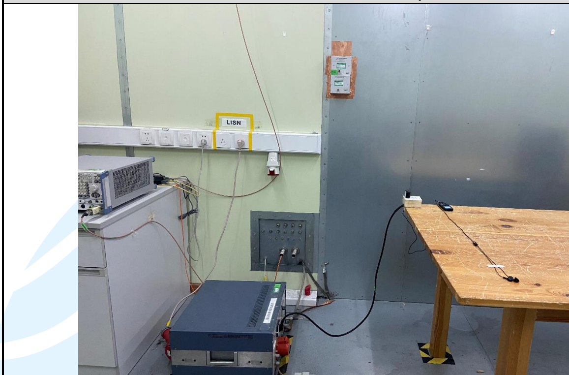
Conducted Emission Test Setup
