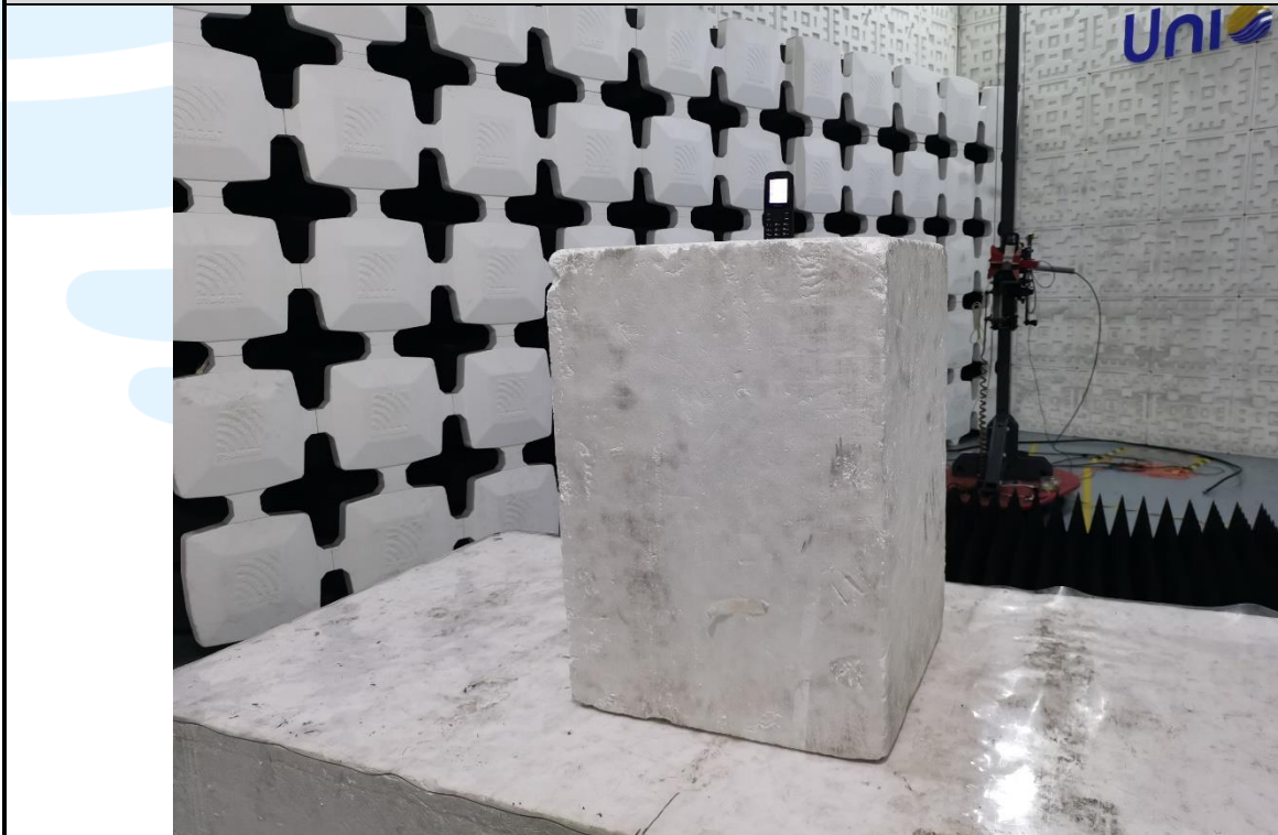
Radiated emission Test Setup (Above 1 GHz)
