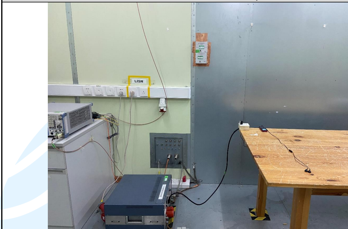
Conducted Emission Test Setup
