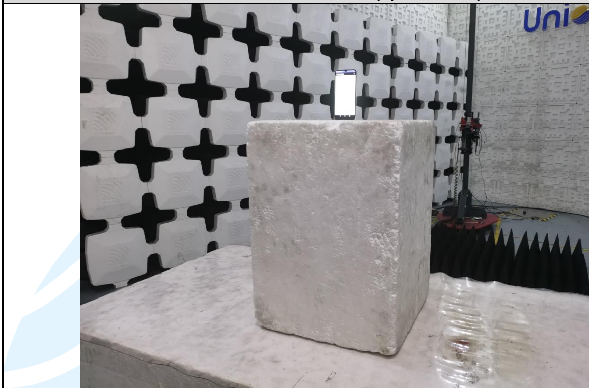
Radiated emission Test Setup (Above 1 GHz)
