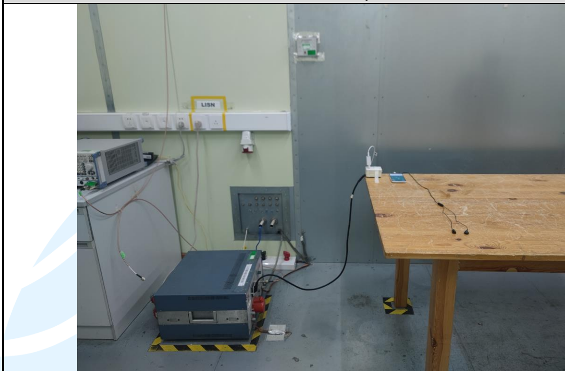
Conducted Emission Test Setup-3 – Test Mode 5
