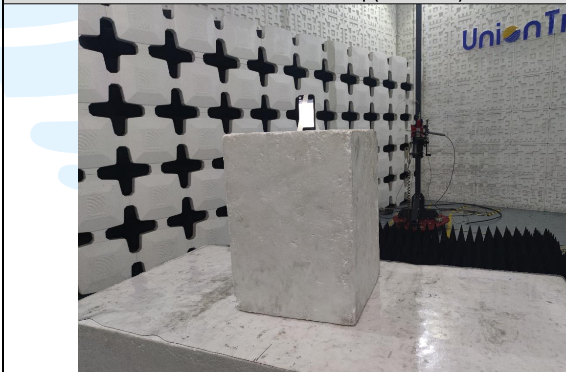
Radiated emission Test Setup (Above 1 GHz)
