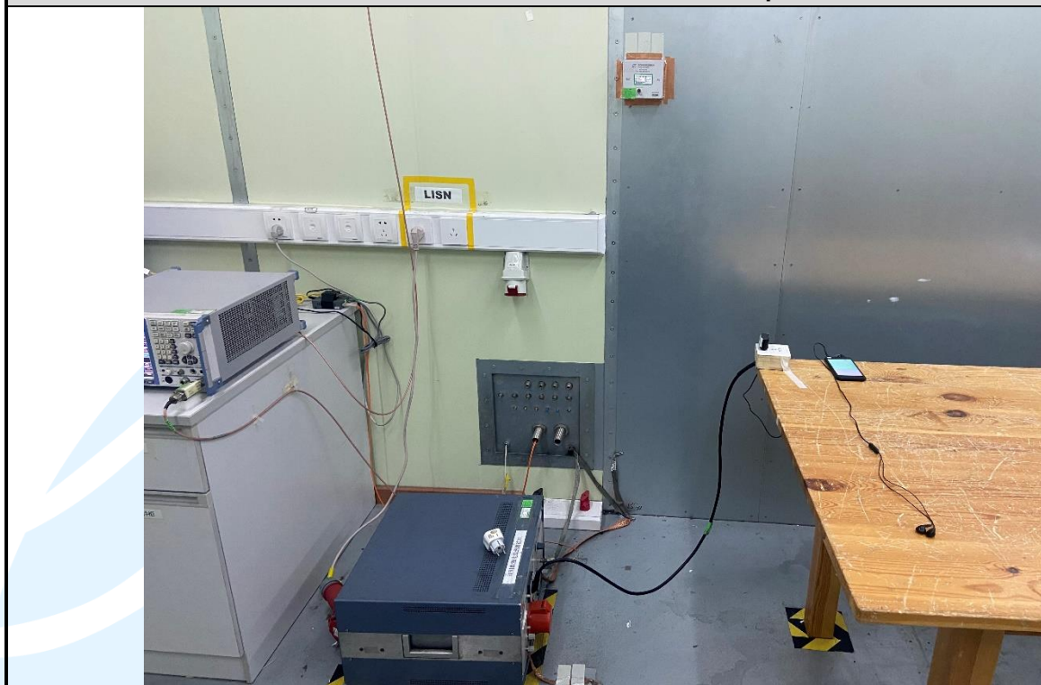
Conducted Emission Test Setup
