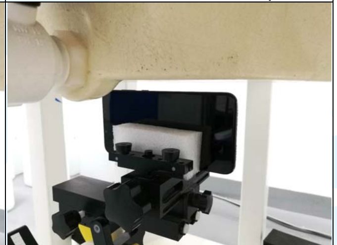
Right Side of EUT with 1.0 cm Gap
