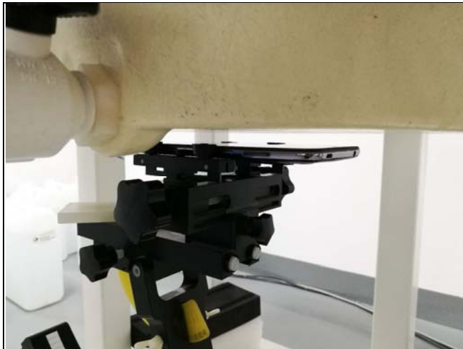
Front Face of EUT with 1.0 cm Gap
