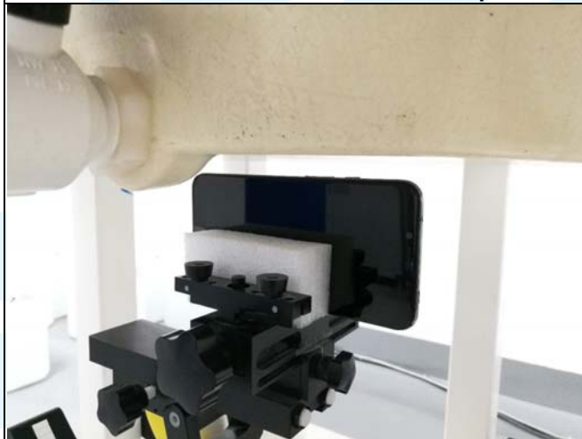
Left Side of EUT with 1.0 cm Gap
