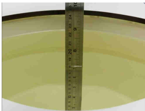
Fig 10.2 Photo of Liquid Height for Body SAR
