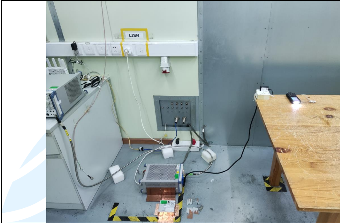
Conducted Emission Test Setup
