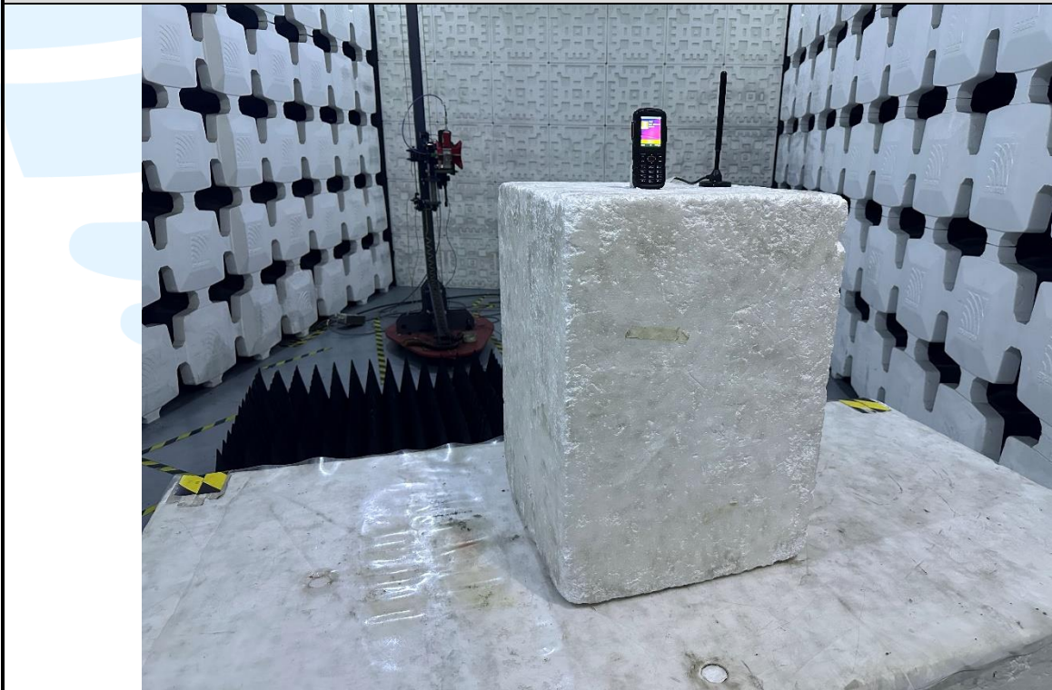
Radiated emission Test Setup (Above 1 GHz)
