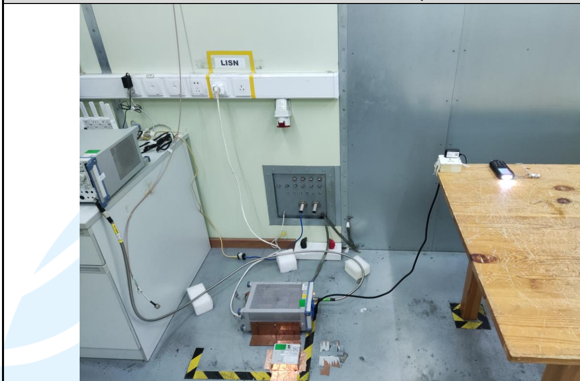
Conducted Emission Test Setup-3
