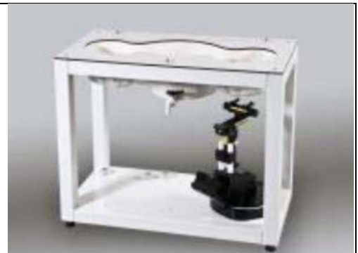
Fig. 6.8 Photo of SAM Phantom
