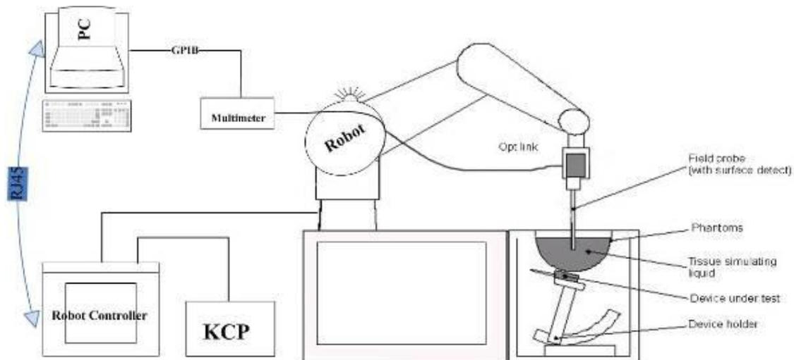
**The OPENSAR system for performing compliance tests consist of the following items:**
