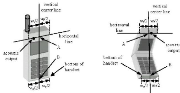
**Figure 6.3 Handset Vertical Center & Horizontal Line Reference Points**
