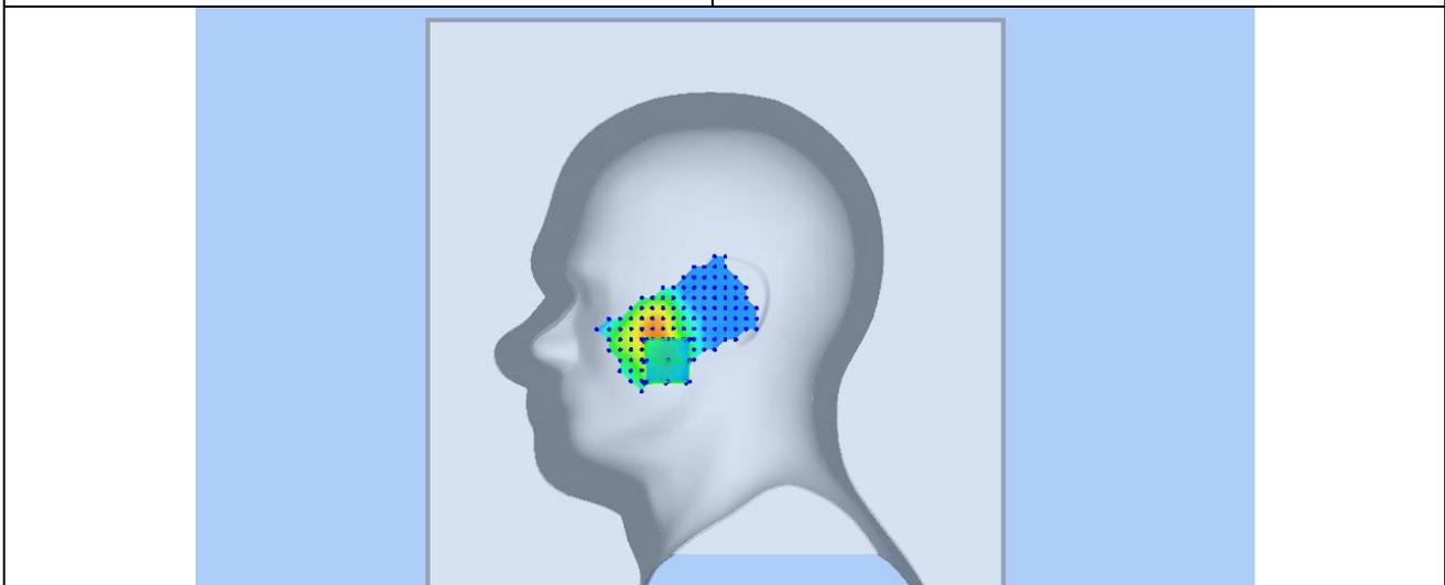
Test mode: WCDMA Band IV, Mid channel (Body Front Side)
