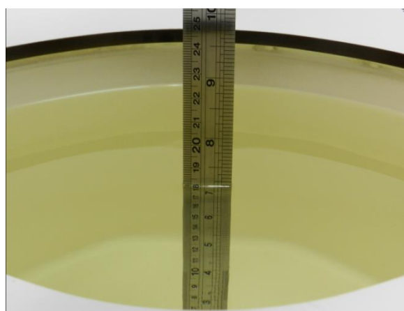
Fig 10.2 Photo of Liquid Height for Body SAR
