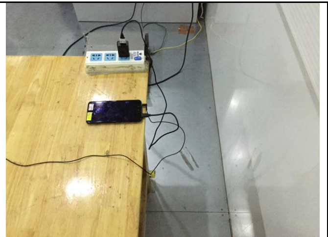
Conducted Emissions Test Setup Side View
