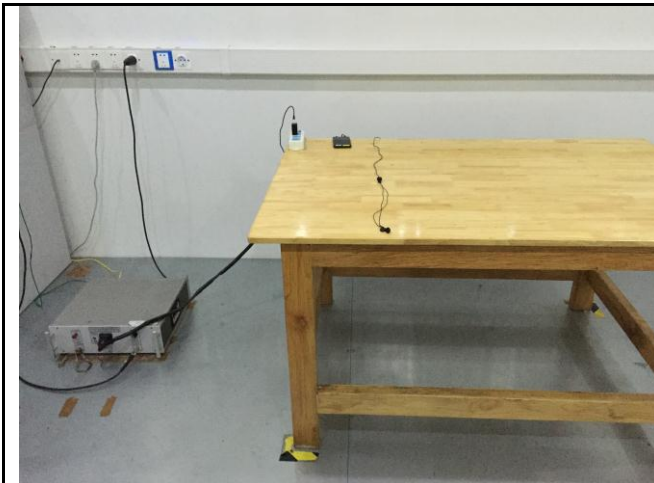
Conducted Emissions Test Setup Front View
