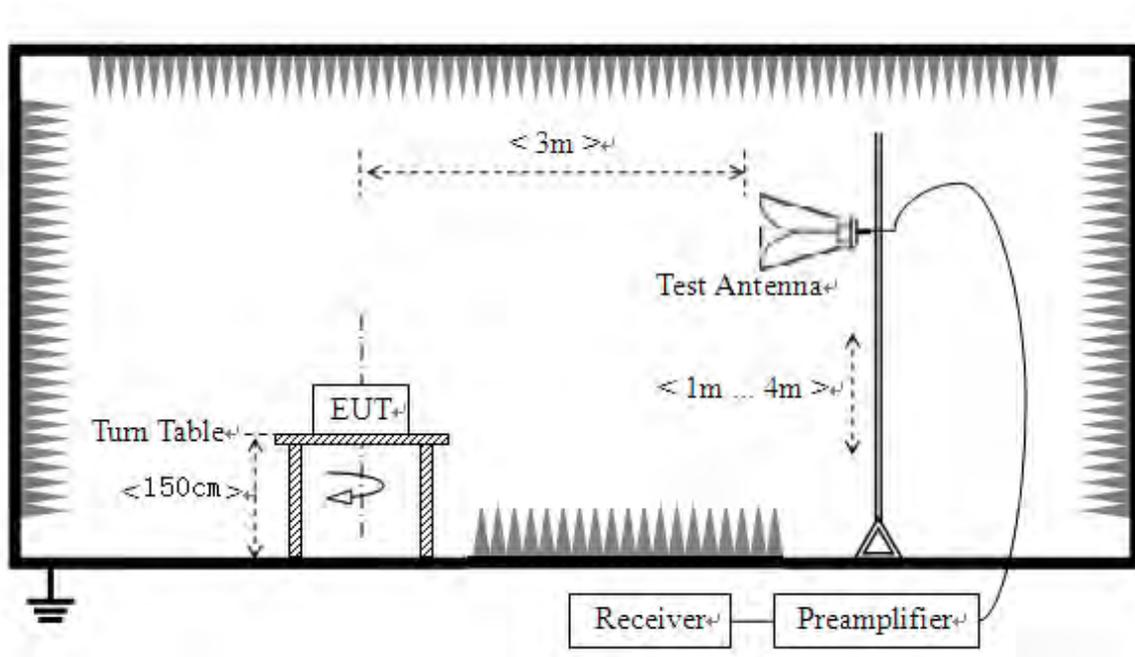
The EUT is placed on a non-conducting table 80 cm above the ground plane for measurement below 1GHz; 1.5 m above the ground plane for measurement above 1GHz. The antenna to EUT distance is 3 meters. The EUT is configured in accordance with ANSI C63.10. The EUT is set to transmit in a continuous mode.
