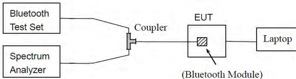
The Bluetooth Module of the EUT is coupled to the Spectrum Analyzer (SA) and the Bluetooth Test Set through the coupler; the RF load attached to the EUT antenna terminal is 50Ohm; the path loss as the factor is calibrated to correct the reading.
