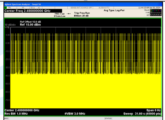
Number of Pulses in 31.6 seconds GFSK_DH3
