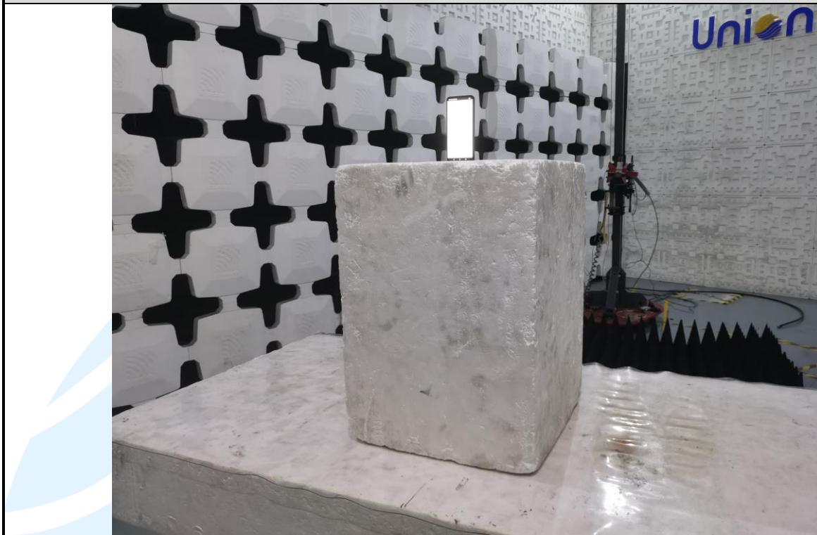
Radiated emission Test Setup (Above 1 GHz)
