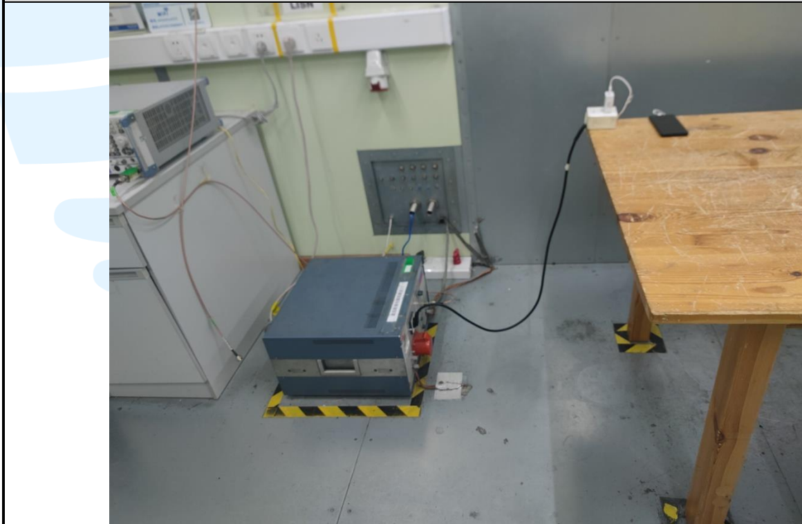
Conducted Emission Test Setup
