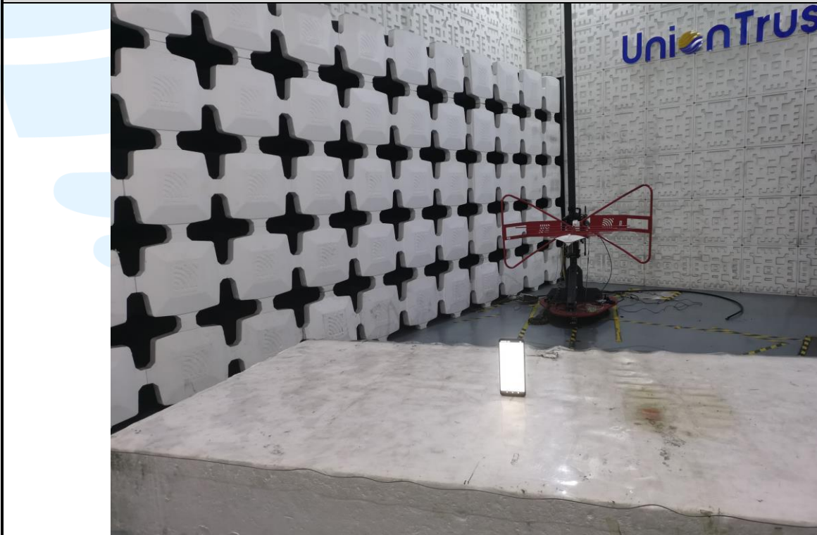
Radiated emission Test Setup (30 MHz~1 GHz)
