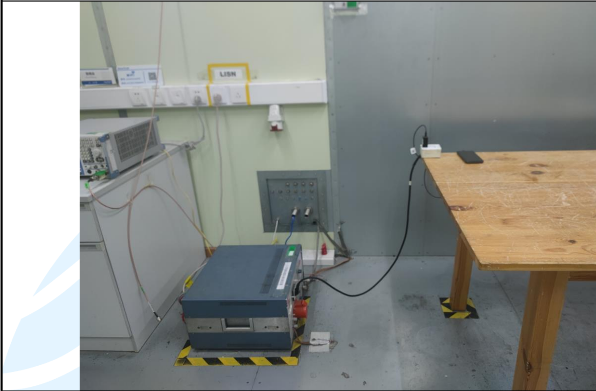
Conducted Emission Test Setup
