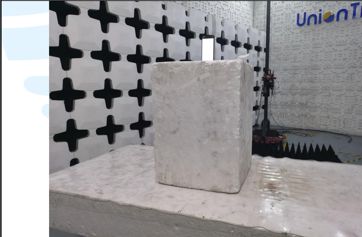
Radiated emission Test Setup (Above 1 GHz)
