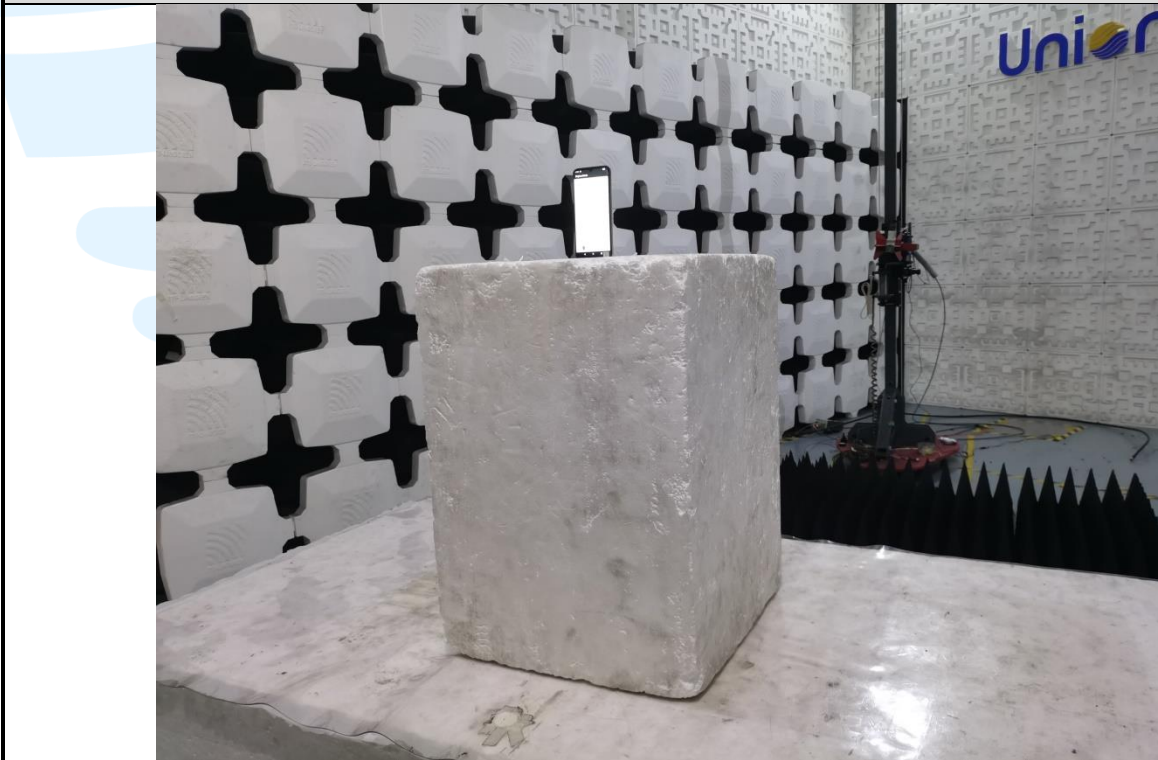
Radiated emission Test Setup (Above 1 GHz)
