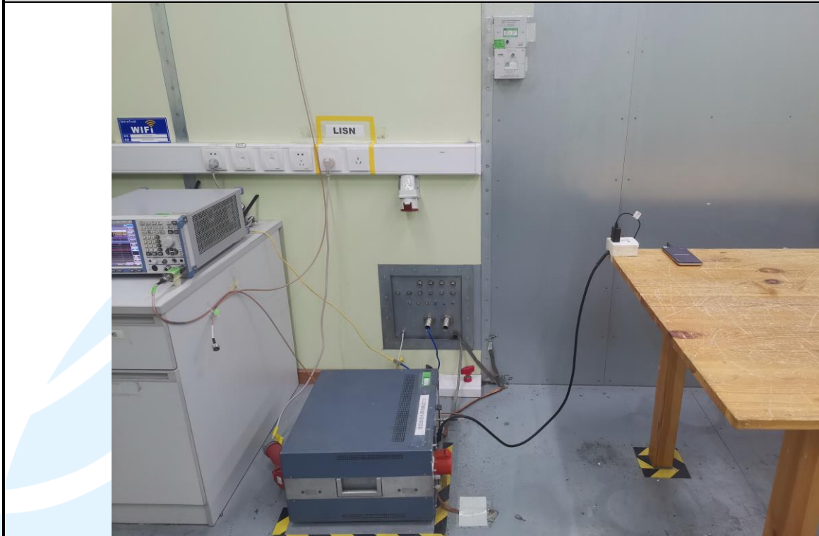
Conducted Emission Test Setup
