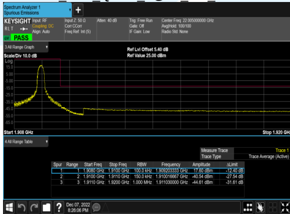
B2 15M 16QAM 1@74 CH 19125
