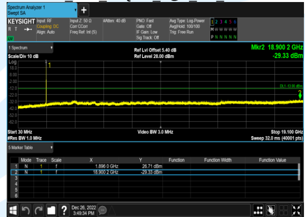
B2 10M 64QAM 1@0 CH 18900
