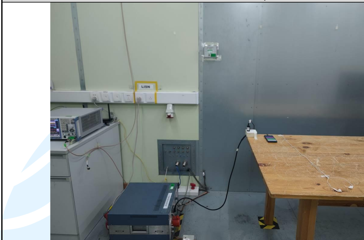
Conducted Emission Test Setup-3
