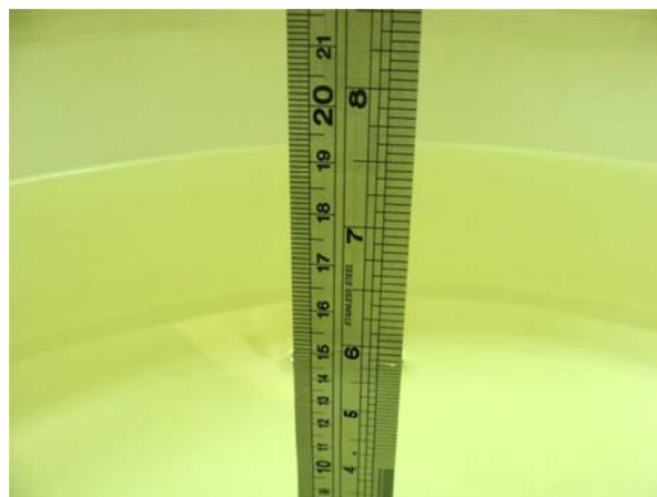
Fig 6.2 Photo of Liquid Height for Body SAR
