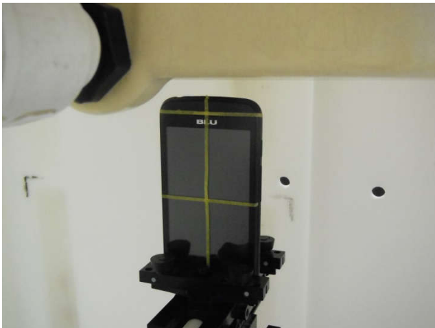
Top Side, Test Separation 10 mm
