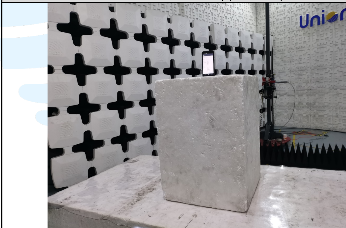
Radiated emission Test Setup (Above 1 GHz)
