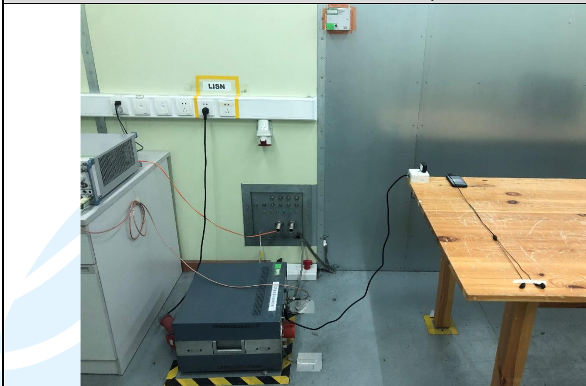
Conducted Emission Test Setup
