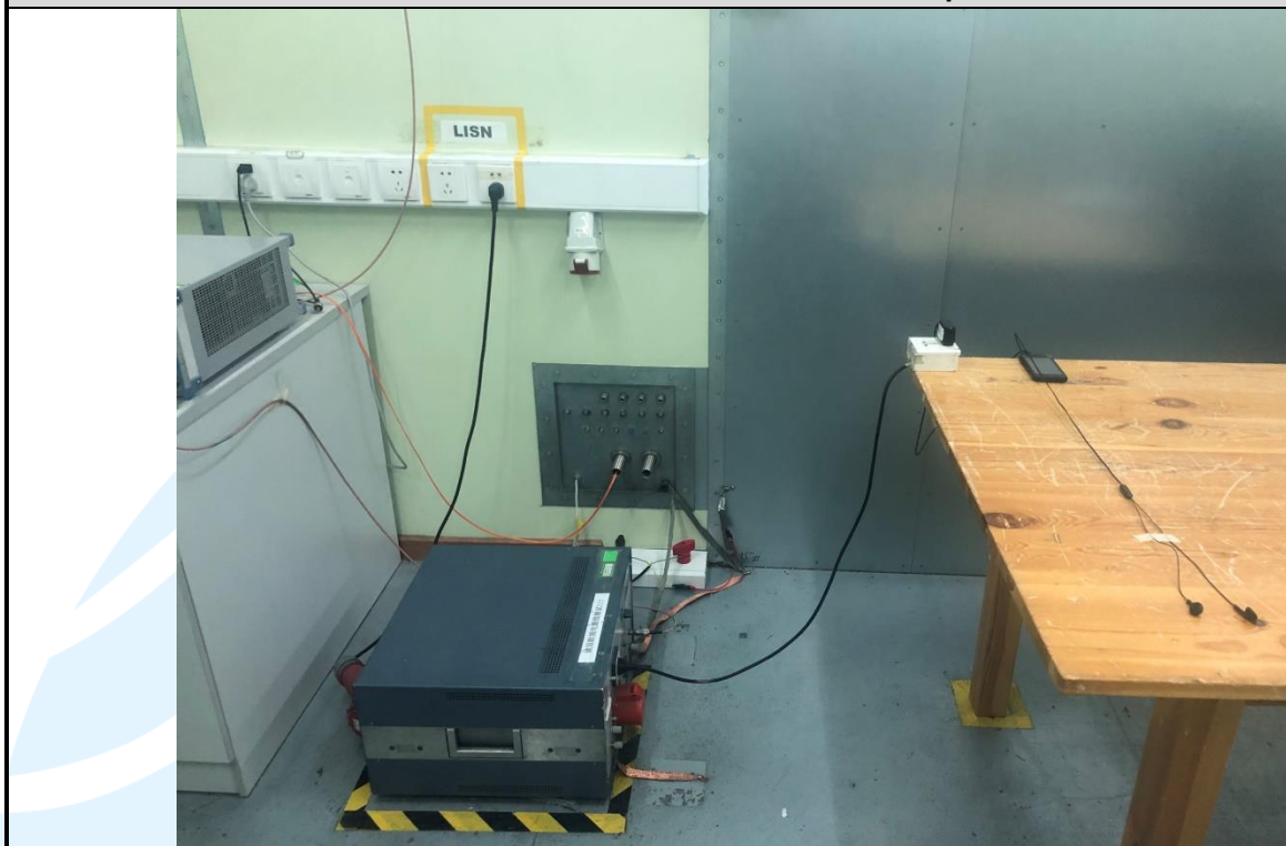
Conducted Emission Test Setup
