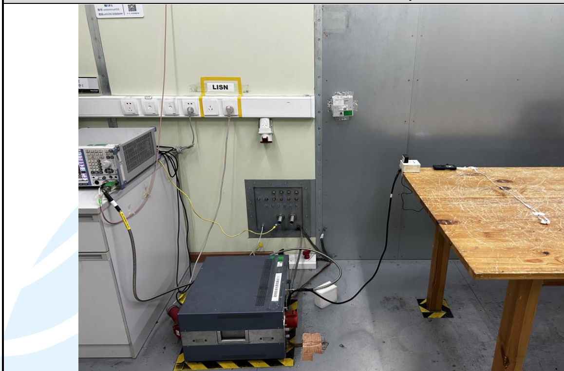
Conducted Emission Test Setup-3
