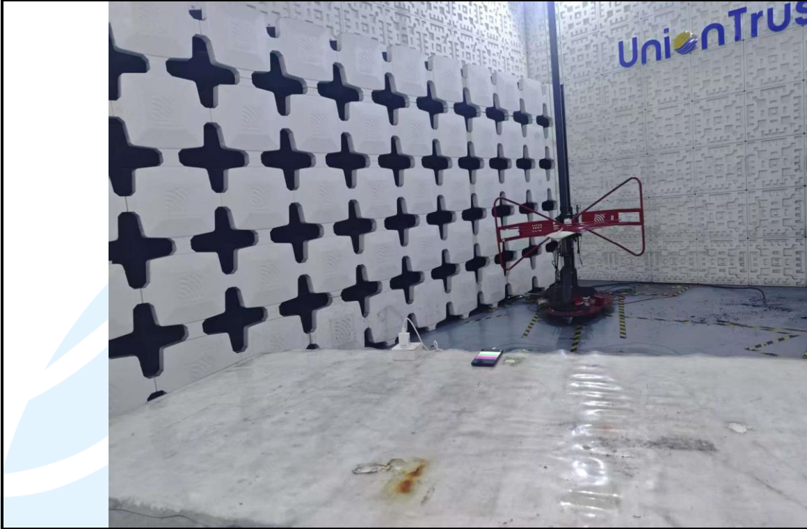
Radiated emission Test Setup-1 (30 MHz~1 GHz)
