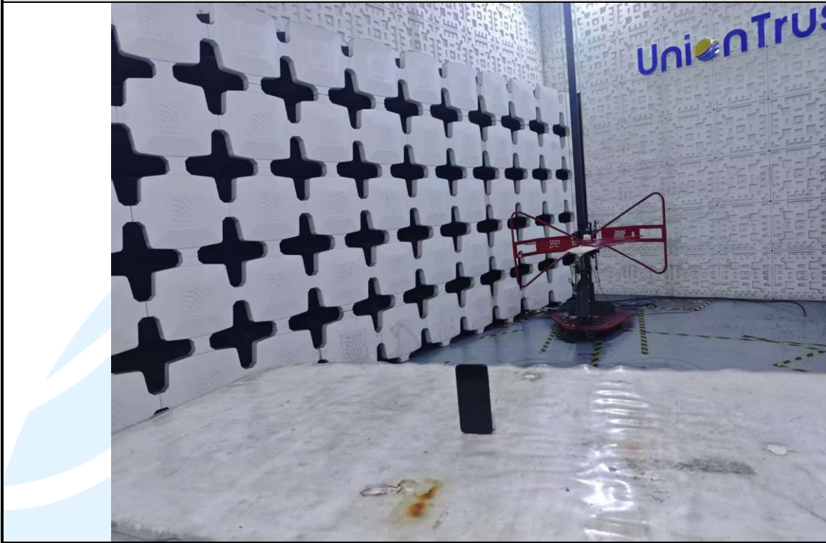
Radiated emission Test Setup (30 MHz~1 GHz)
