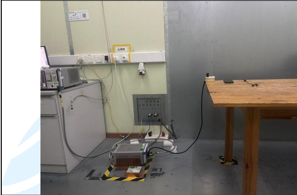
Conducted Emission Test Setup
