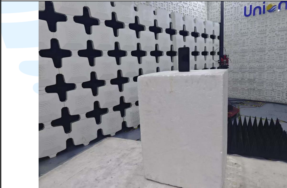
Radiated emission Test Setup (Above 1 GHz)
