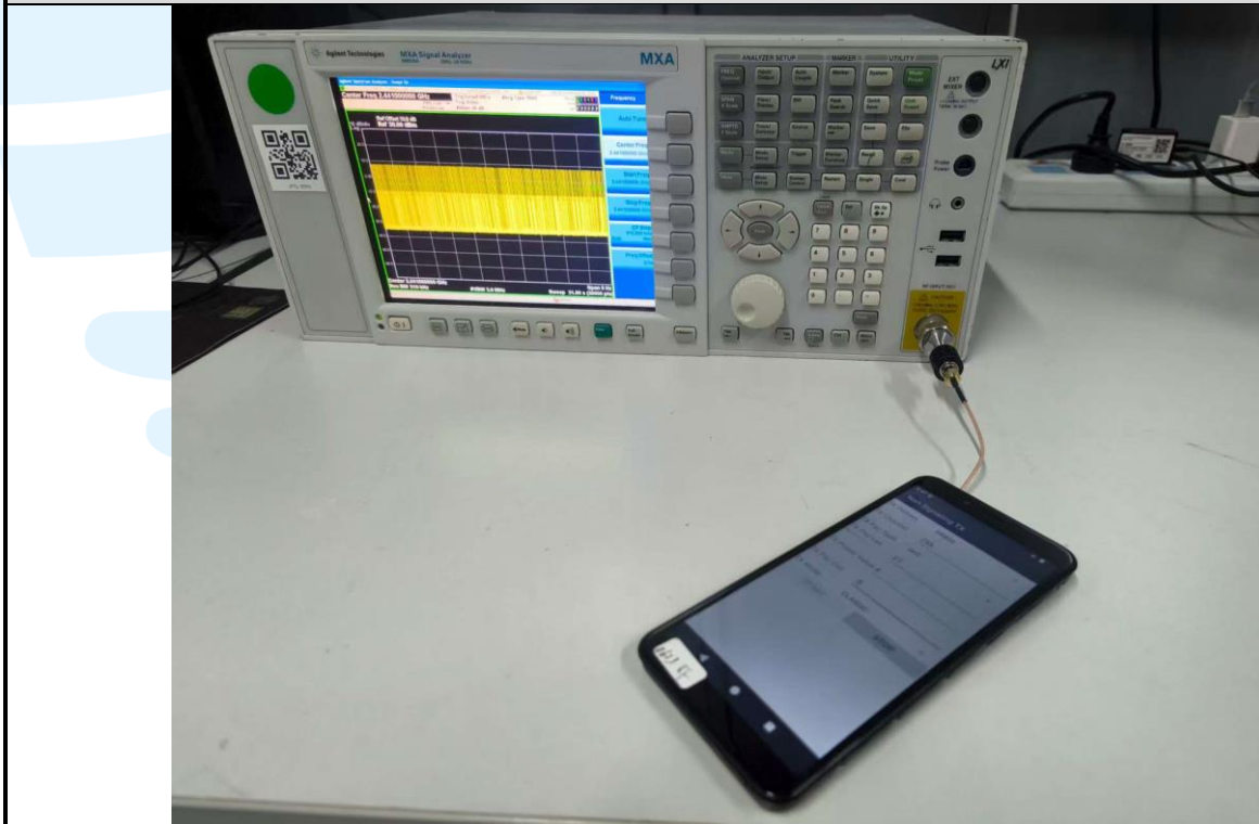
RF Conducted Test Setup
