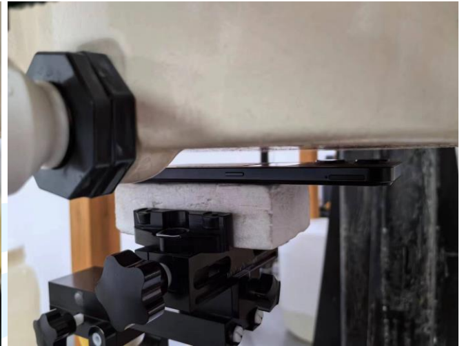
Rear Face of EUT with 1 cm Gap
