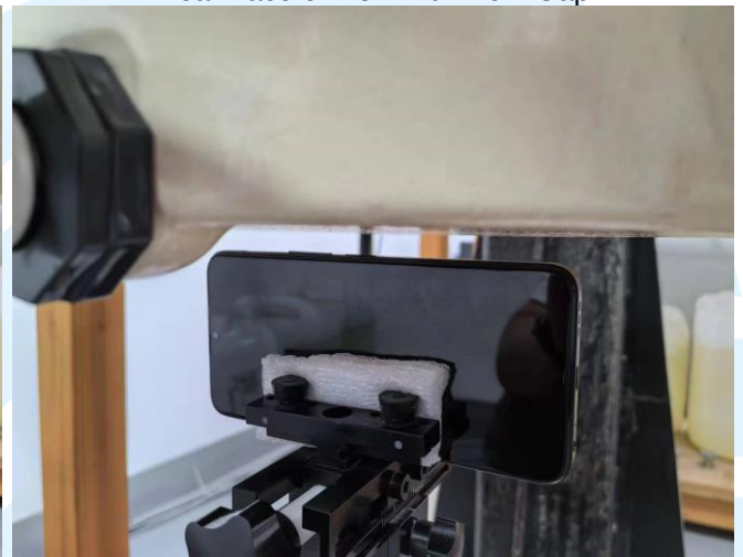
Right Side of EUT with 1 cm Gap
