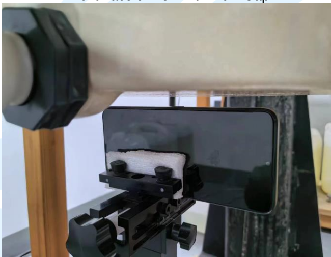
Left Side of EUT with 1 cm Gap
