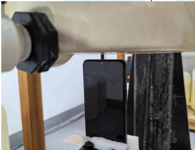
Top Side of EUT with 1 cm Gap
