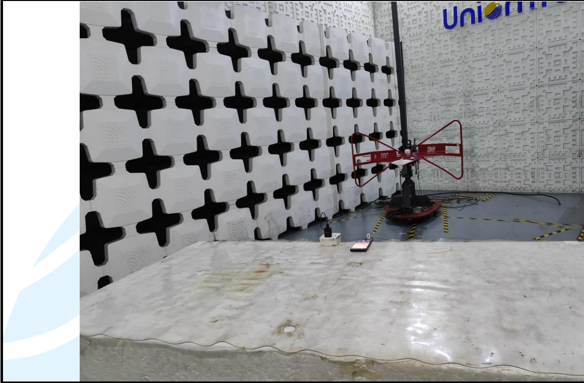
Radiated emission Test Setup (30 MHz~1 GHz)
