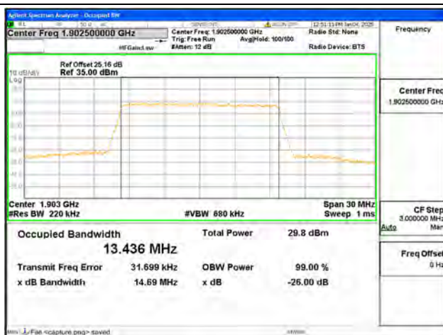
B2 / 15MHz / QPSK/ High CH
