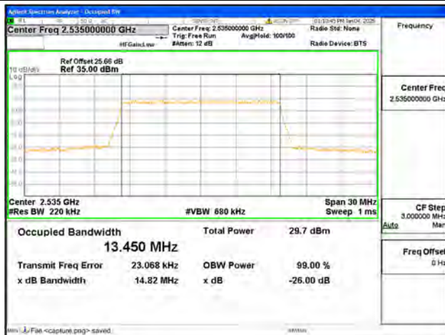
B7 / 15MHz / QPSK/ Mid CH
