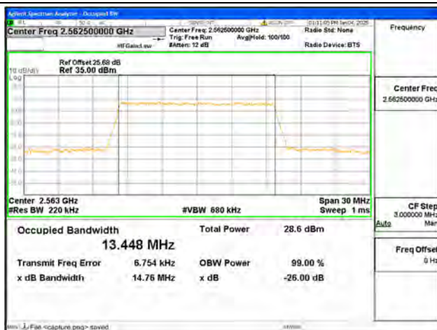
B7 / 15MHz / QPSK/ High CH
