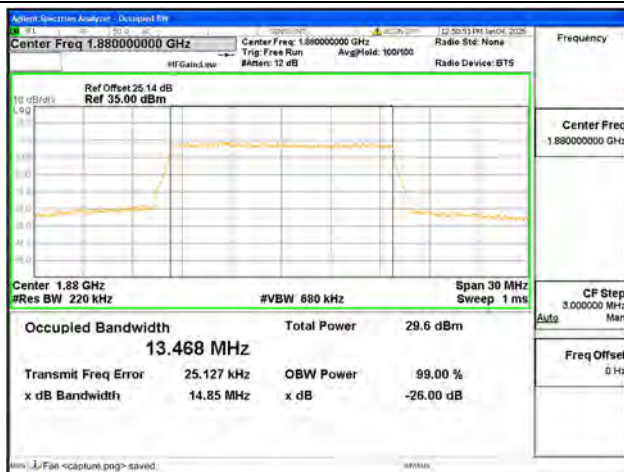
B2 / 15MHz / QPSK/ Mid CH
