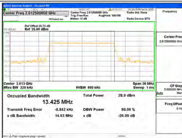
B38 / 15MHz / QPSK/ High CH
