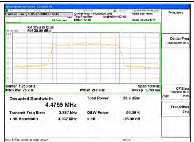
B2 / 5MHz / 16QAM/ Low CH
