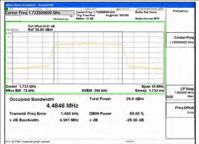
B4 / 5MHz / 16QAM/ Mid CH
