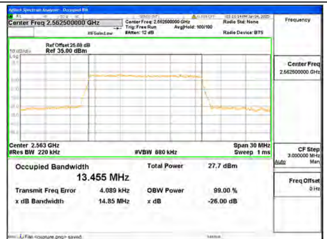
B7 / 15MHz / 16QAM/ High CH
