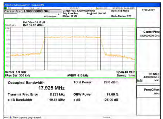
B2 / 20MHz / 16QAM/ High CH
