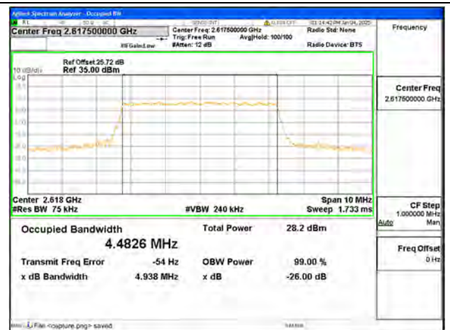
B38 / 5MHz / 16QAM/ High CH
