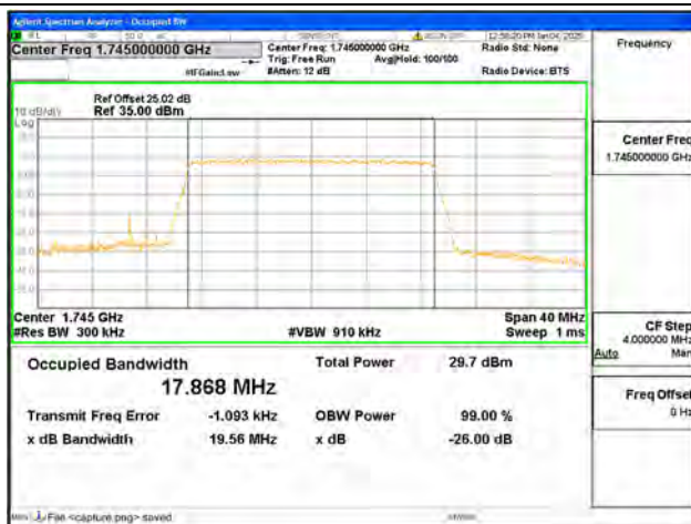
B4 / 20MHz / QPSK/ High CH
