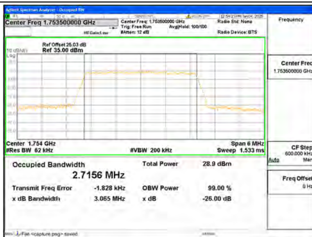
B4 / 3MHz / QPSK/ High CH
