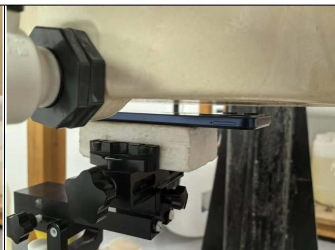
Rear Face of EUT with 1.0 cm Gap
