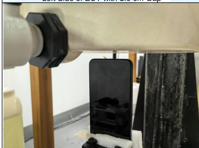
Bottom Side of EUT with 1.0 cm Gap
