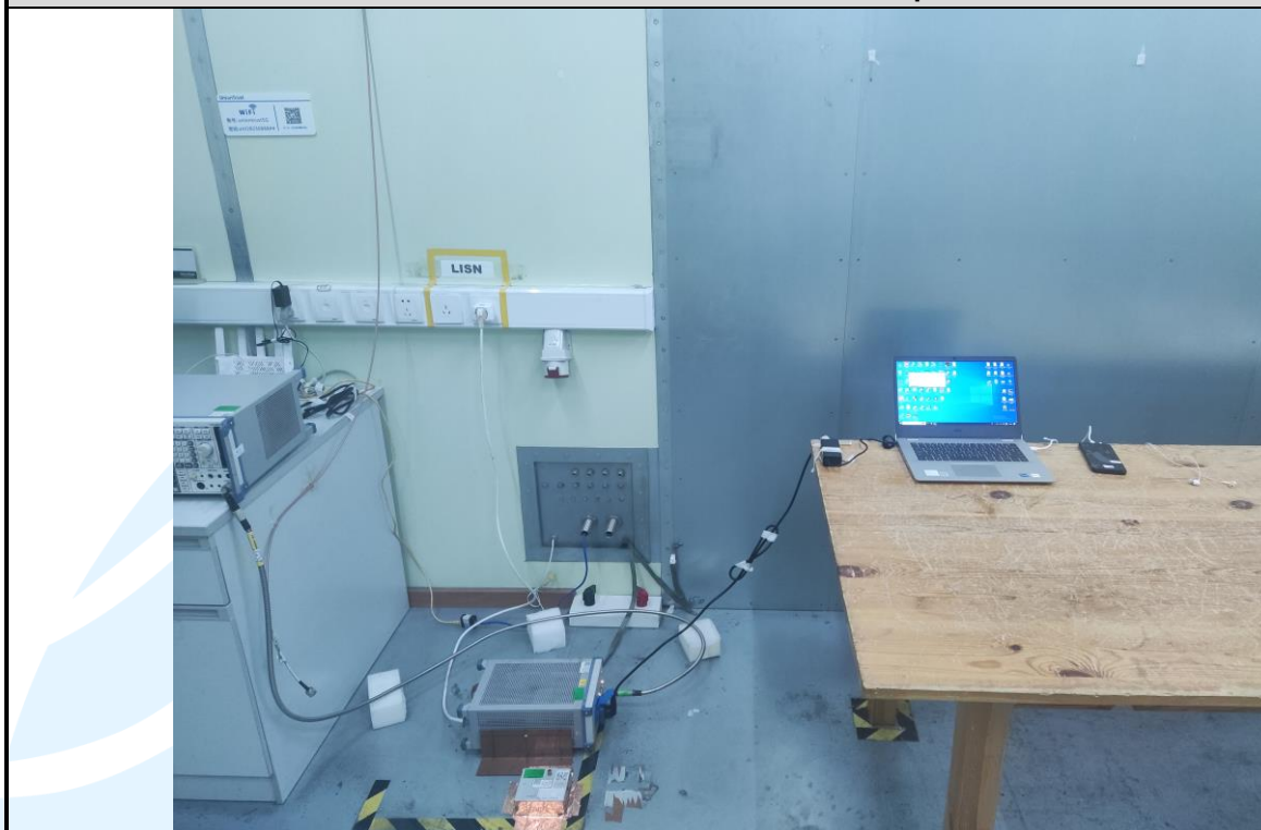
Conducted Emission Test Setup-3
