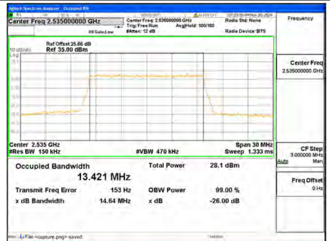
B7 / 15MHz / QPSK/ Mid CH
