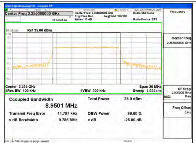
B40-2 / 10MHz / 64QAM/ Mid CH
