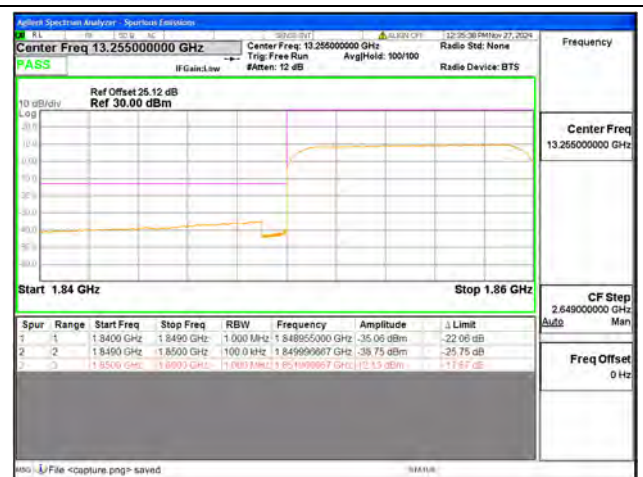
B2 / 10MHz / Low CH / QPSK / FULL RB
