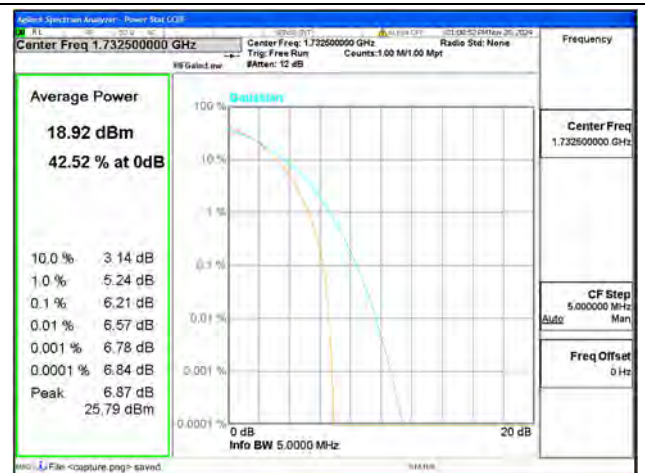
B4 / 1.4MHz / Mid CH / 64QAM
