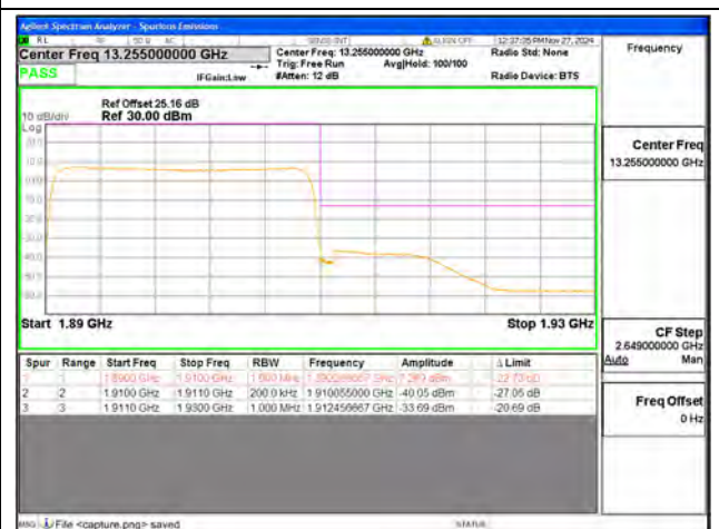
B2 / 20MHz / High CH / QPSK / FULL RB
