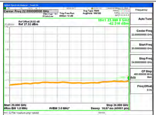
B40-2-20G-24G / 5MHz / Low CH / QPSK
