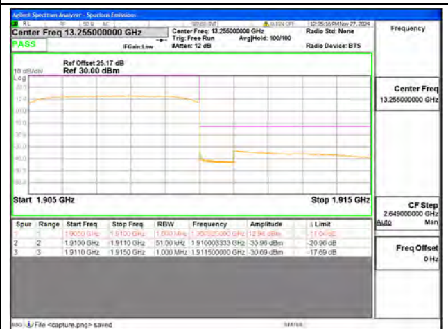
B2 / 5MHz / High CH / QPSK / FULL RB
