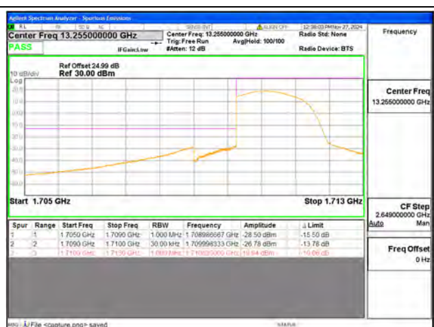
B4 / 1.4MHz / Low CH / QPSK / FULL RB
