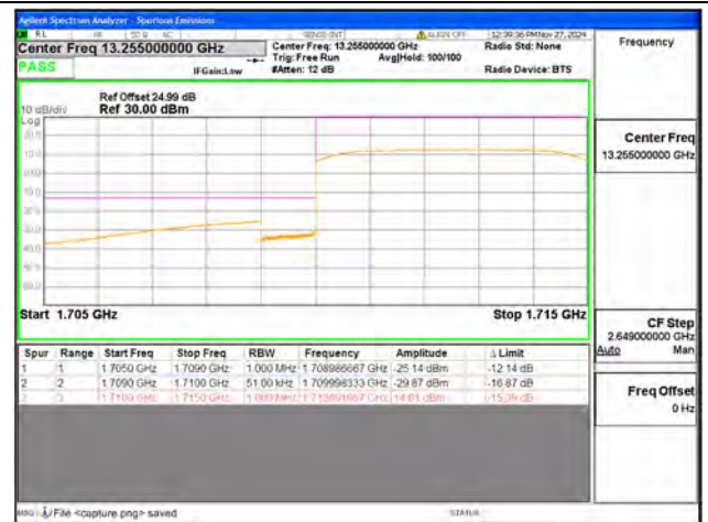
B4 / 5MHz / Low CH / QPSK / FULL RB
