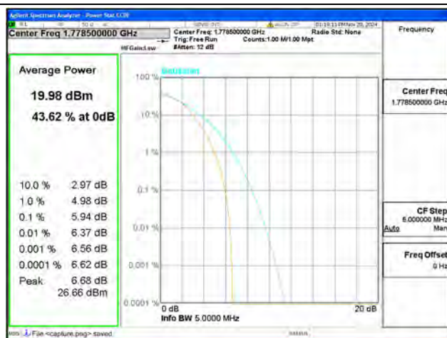
B66 / 3MHz / High CH / 16QAM
