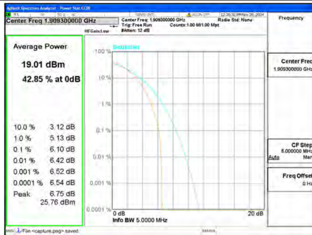
B2 / 1.4MHz / High CH / 64QAM
