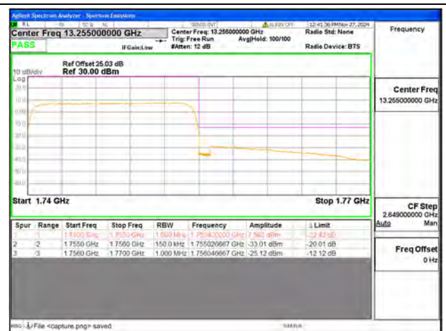
B4 / 15MHz / High CH / QPSK / FULL RB
