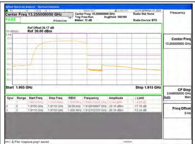
B2 / 3MHz / High CH / QPSK / FULL RB
