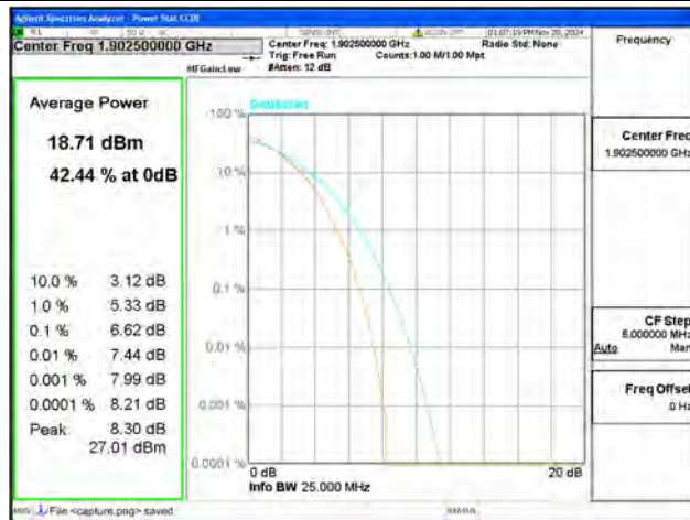
B2 / 15MHz / High CH / 64QAM
