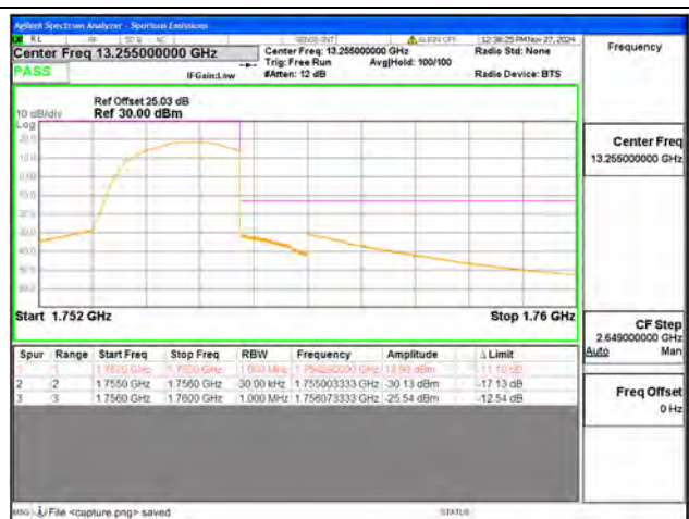
B4 / 1.4MHz / High CH / QPSK / FULL RB
