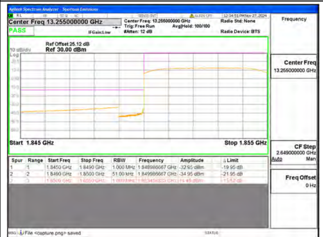
B2 / 5MHz / Low CH / QPSK / FULL RB
