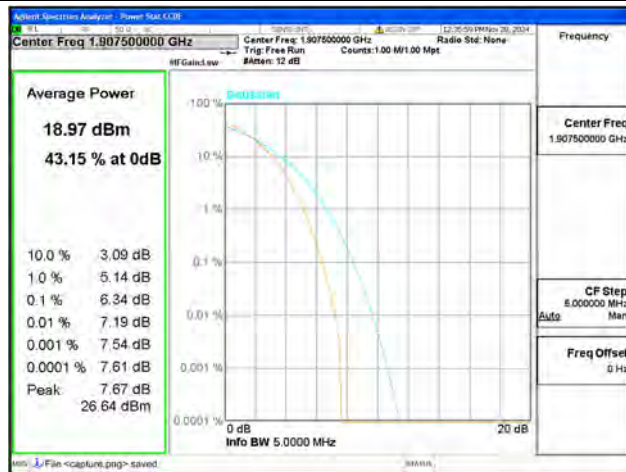
B2 / 5MHz / High CH / 64QAM
