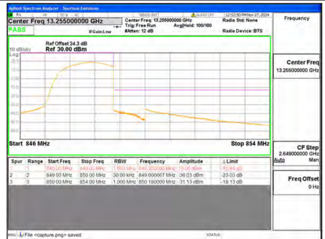
B5 / 1.4MHz / High CH / QPSK / FULL RB
