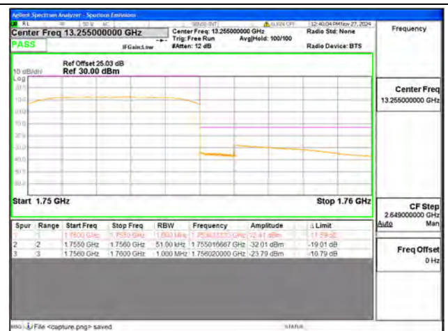
B4 / 5MHz / High CH / QPSK / FULL RB
