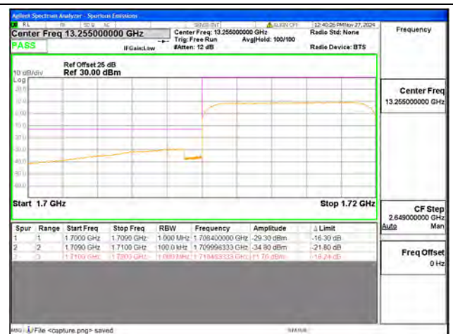
B4 / 10MHz / Low CH / QPSK / FULL RB
