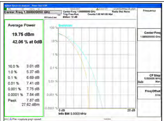
B2 / 3MHz / Mid CH / 16QAM
