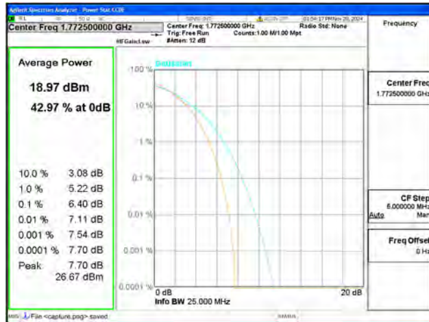
B66 / 15MHz / High CH / 64QAM
