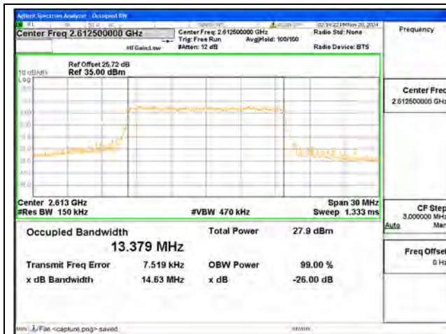
B38 / 15MHz / QPSK/ High CH
