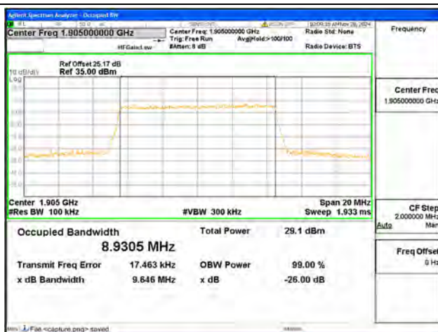
B2 / 10MHz / 16QAM/ High CH
