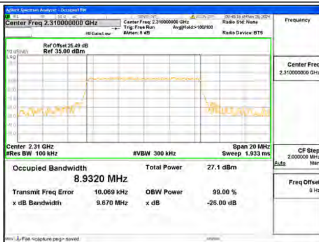
B40-1 / 10MHz / 16QAM/ Mid CH
