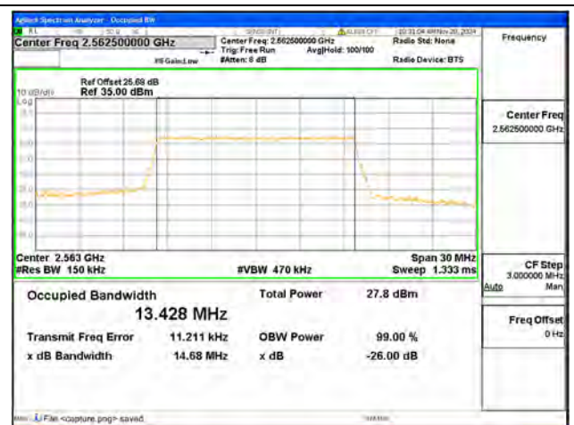
B7 / 15MHz / 16QAM/ High CH
