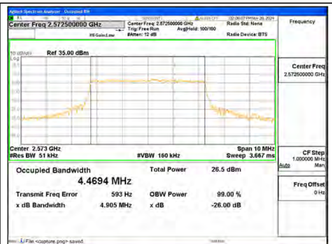
B38 / 5MHz / 16QAM/ Low CH
