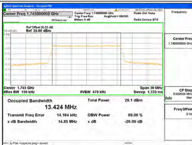
B66 / 15MHz / 16QAM/ Mid CH
