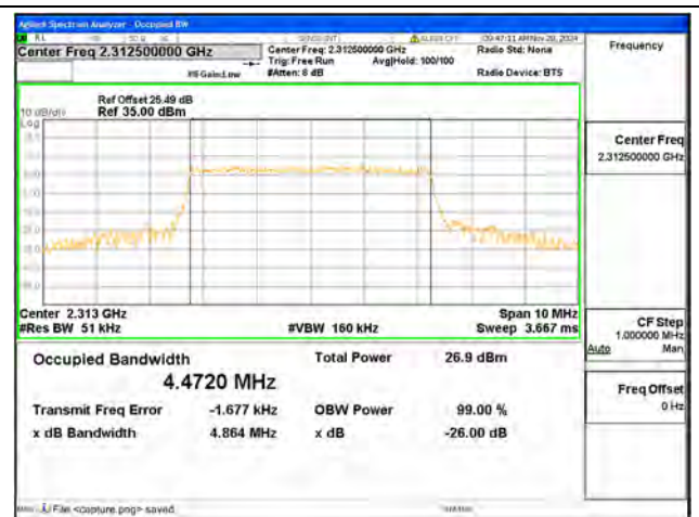
B40-1 / 5MHz / 16QAM/ High CH
