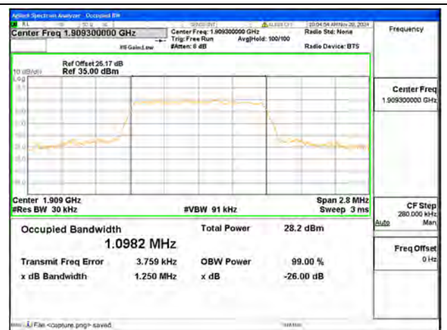
B2 / 1.4MHz / 16QAM/ High CH
