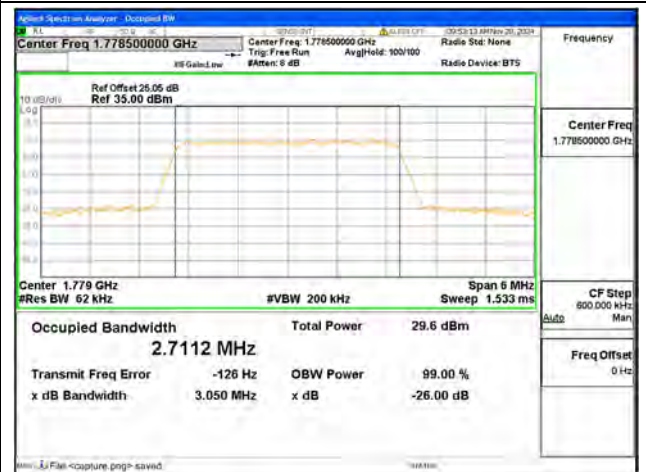
B66 / 3MHz / QPSK/ High CH
