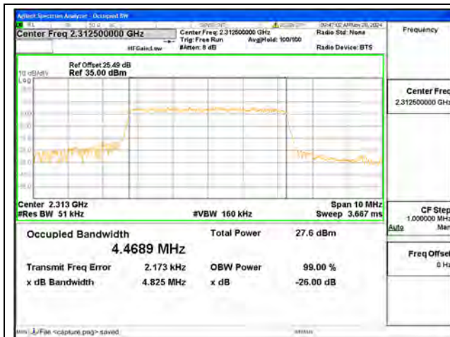
B40-1 / 5MHz / QPSK/ High CH
