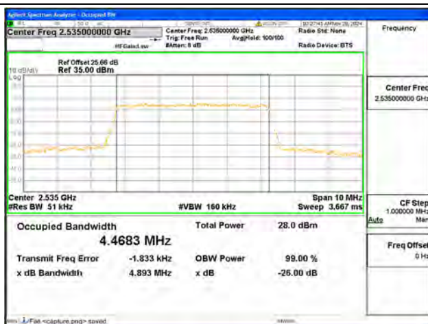
B7 / 5MHz / 16QAM/ Mid CH
