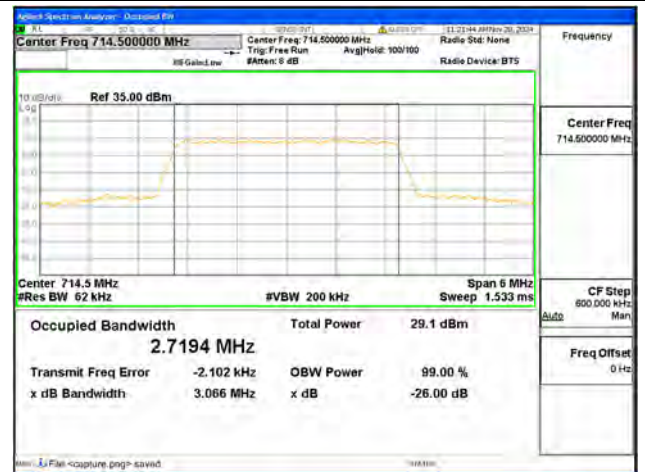
B12 / 3MHz / QPSK/ High CH
