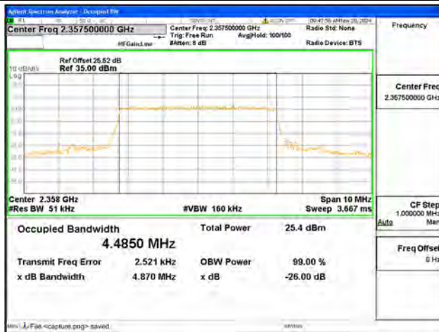
B40-2 / 5MHz / 64QAM/ High CH
