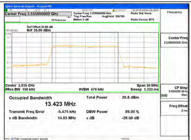
B7 / 15MHz / 64QAM/ Mid CH
