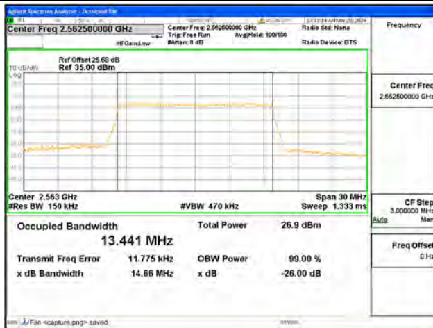
B7 / 15MHz / 64QAM/ High CH
