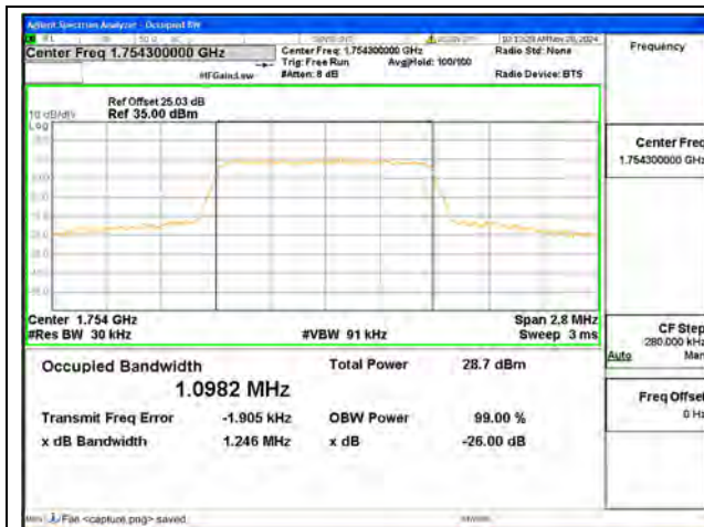
B4 / 1.4MHz / QPSK/ High CH
