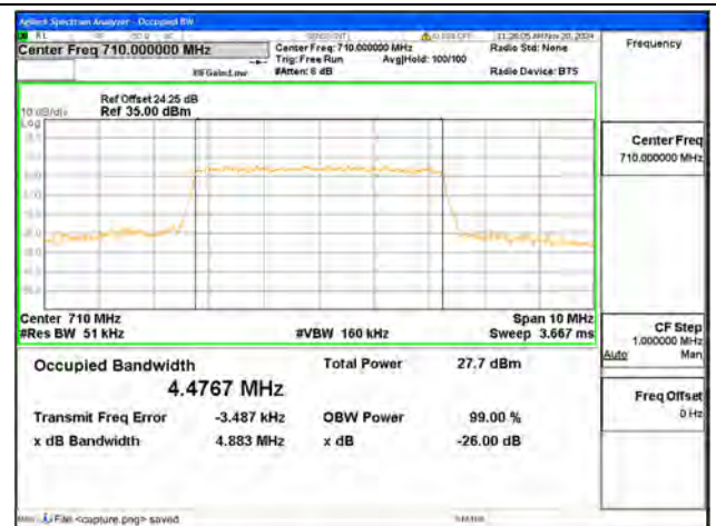
B17 / 5MHz / 64QAM/ Mid CH
