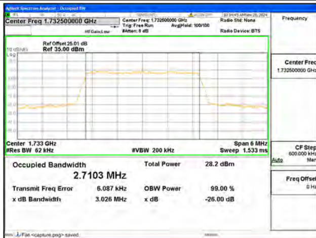
B4 / 3MHz / 64QAM/ Mid CH
