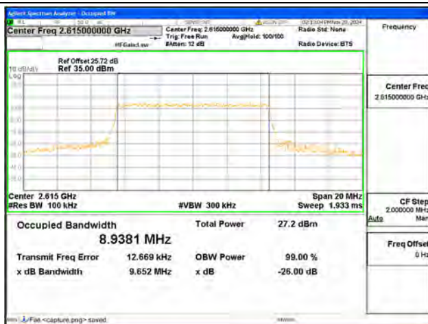
B38 / 10MHz / 16QAM/ High CH
