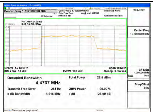
B4 / 5MHz / 16QAM/ Low CH
