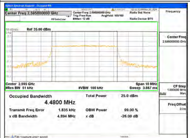
B38 / 5MHz / 64QAM/ Mid CH
