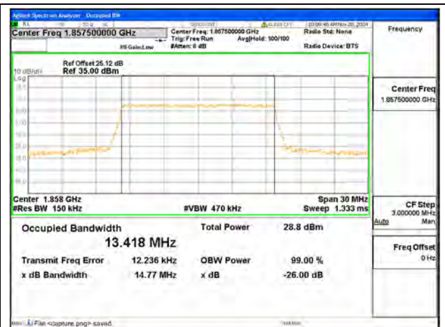
B2 / 15MHz / 16QAM/ Low CH
