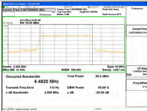
B7 / 5MHz / 64QAM/ High CH
