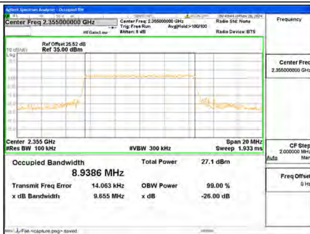
B40-2 / 10MHz / 16QAM/ Mid CH
