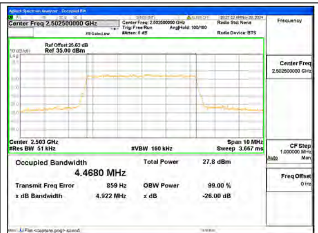
B7 / 5MHz / 16QAM/ Low CH
