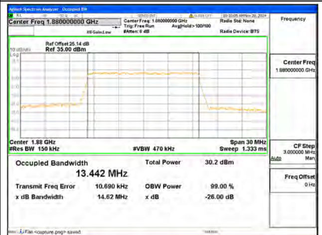
B2 / 15MHz / QPSK/ Mid CH
