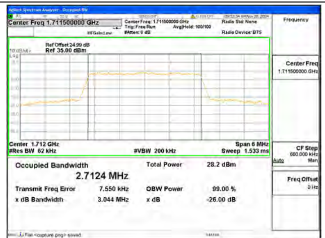
B66 / 3MHz / 64QAM/ Low CH
