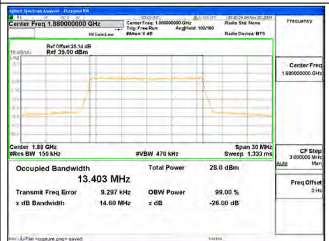
B2 / 15MHz / 64QAM/ Mid CH
