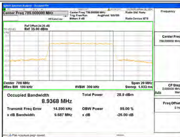
B17 / 10MHz / 16QAM/ Low CH
