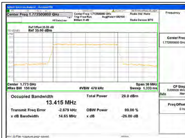
B66 / 15MHz / QPSK/ High CH
