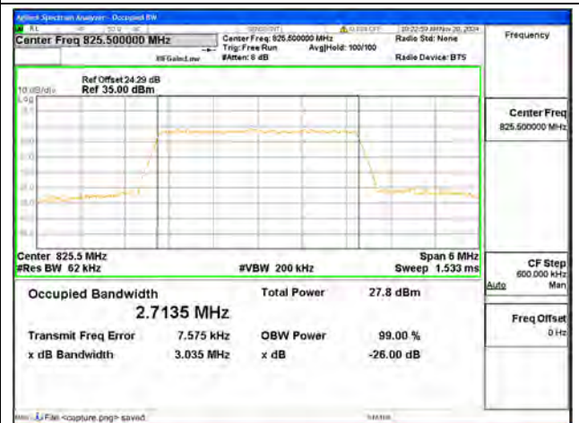
B5 / 3MHz / 64QAM/ Low CH
