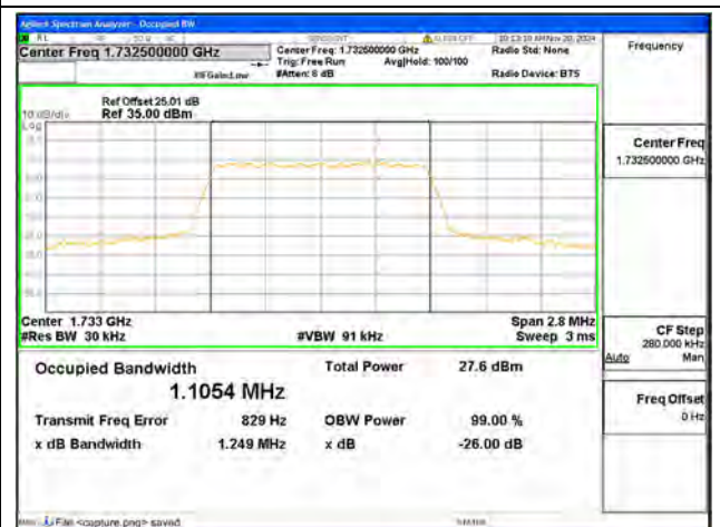
B4 / 1.4MHz / 64QAM/ Mid CH
