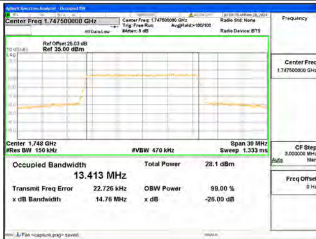
B4 / 15MHz / 64QAM/ High CH
