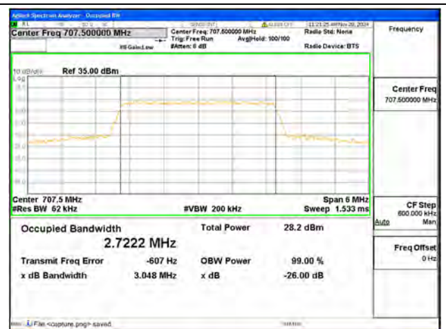
B12 / 3MHz / 16QAM/ Mid CH
