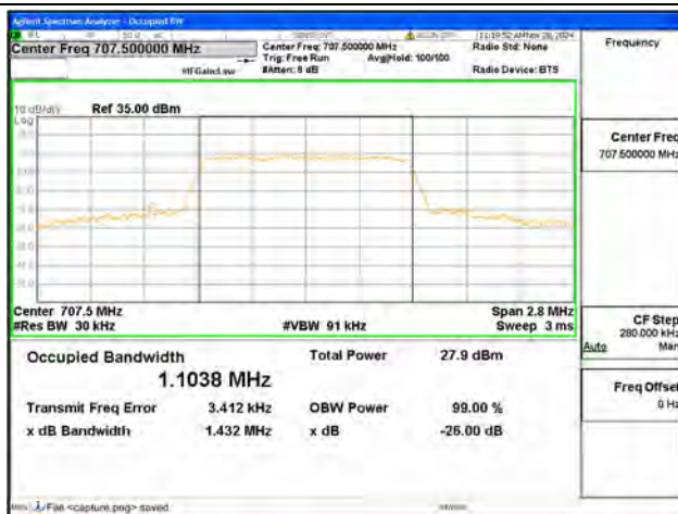
B12 / 1.4MHz / 16QAM/ Mid CH
