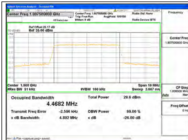
B2 / 5MHz / QPSK/ High CH
