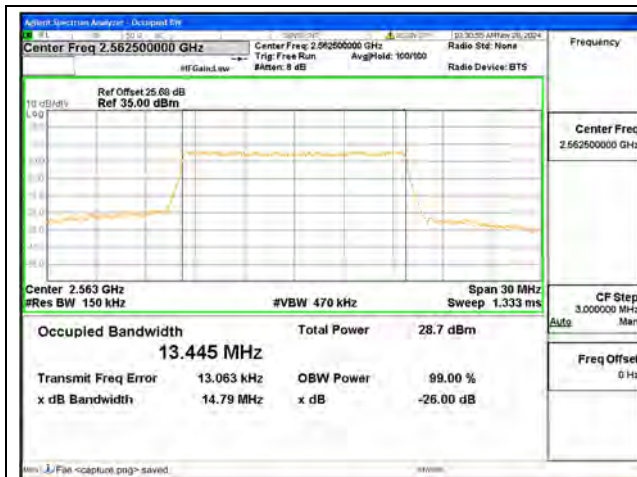
B7 / 15MHz / QPSK/ High CH
