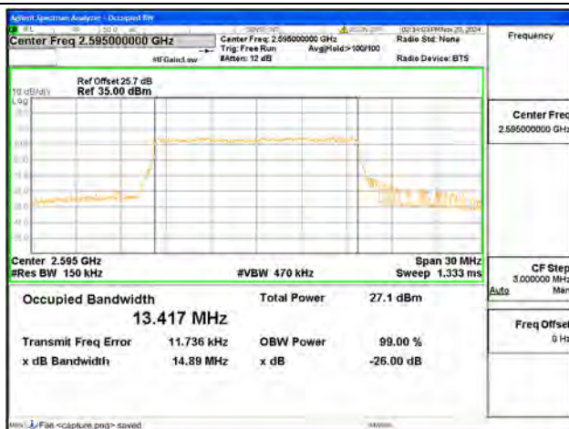
B38 / 15MHz / 16QAM/ Mid CH
