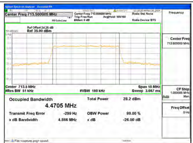
B17 / 5MHz / 16QAM/ High CH
