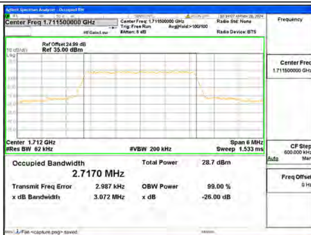
B4 / 3MHz / 16QAM/ Low CH
