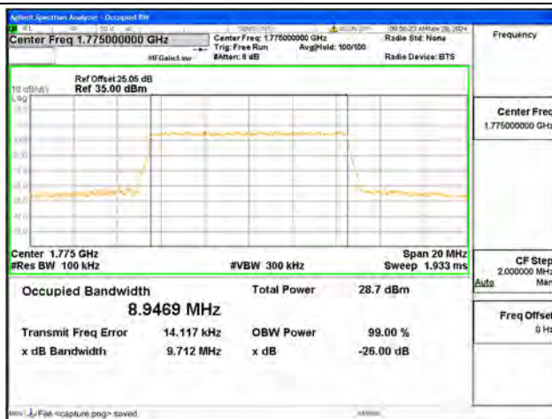
B66 / 10MHz / 16QAM/ High CH
