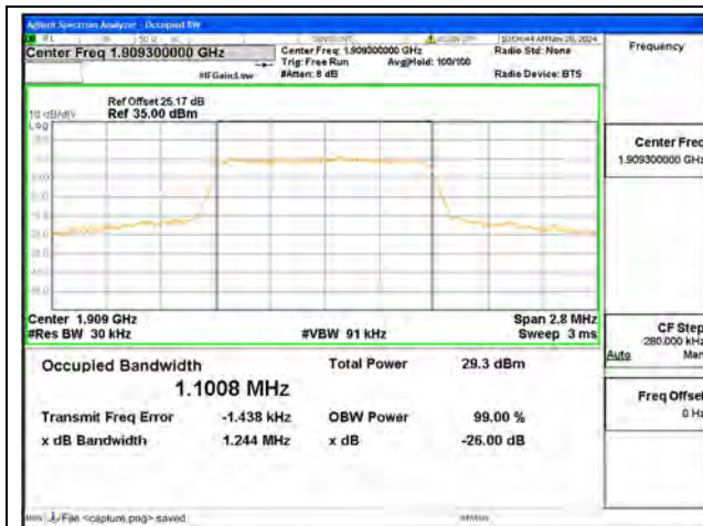
B2 / 1.4MHz / QPSK/ High CH
