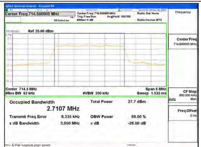
B12 / 3MHz / 64QAM/ High CH
