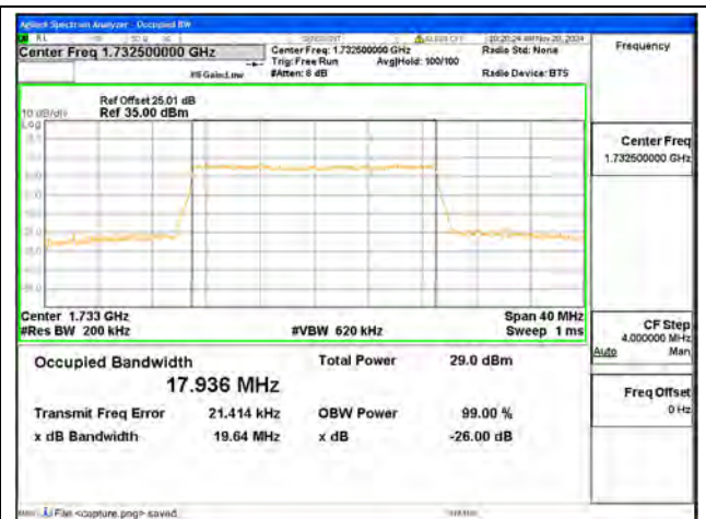
B4 / 20MHz / 16QAM/ Mid CH
