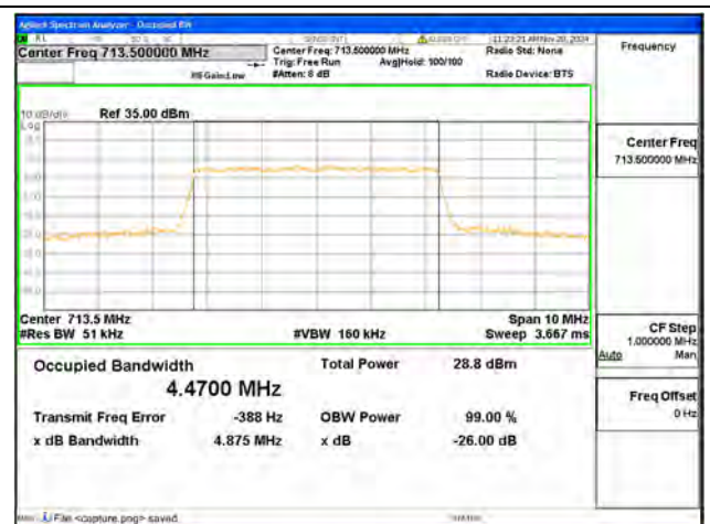
B12 / 5MHz / 16QAM/ High CH
