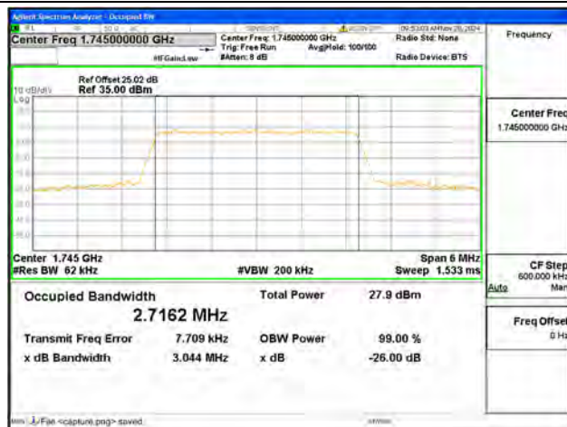
B66 / 3MHz / 64QAM/ Mid CH
