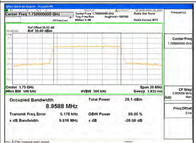
B4 / 10MHz / 64QAM/ High CH
