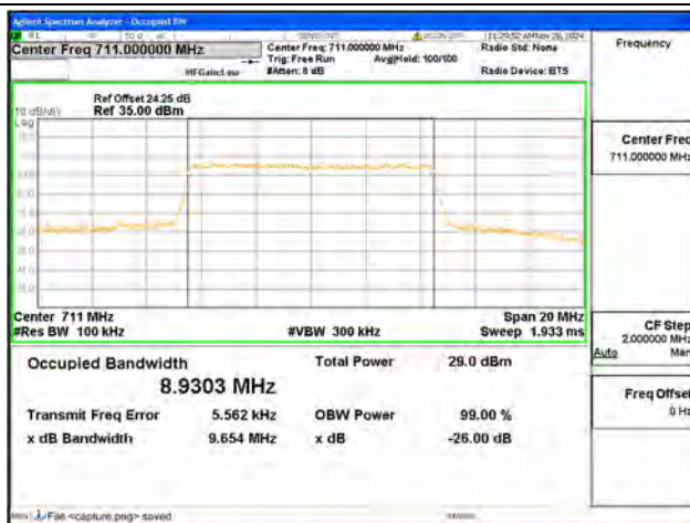
B17 / 10MHz / 16QAM/ High CH
