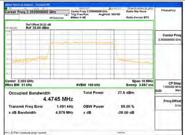
B40-2 / 5MHz / QPSK/ Mid CH
