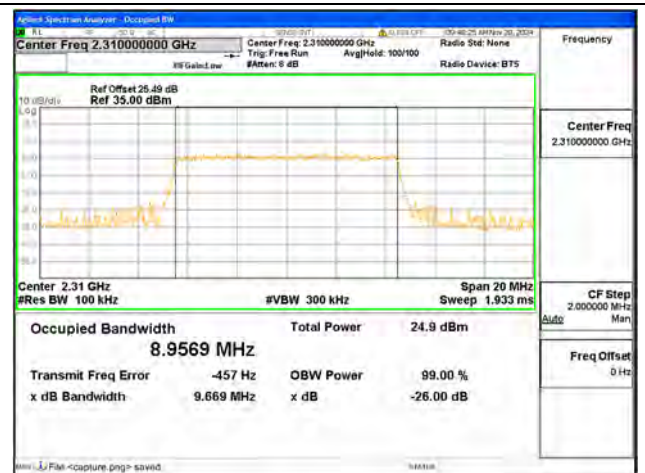
B40-1 / 10MHz / 64QAM/ Mid CH
