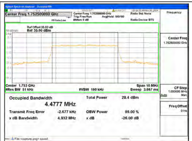
B4 / 5MHz / 16QAM/ High CH
