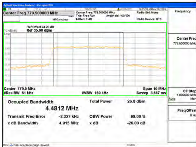
B13 / 5MHz / 64QAM/ Low CH
