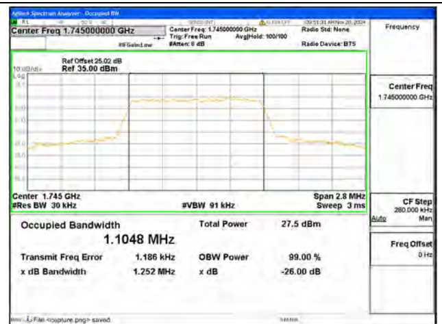
B66 / 1.4MHz / 64QAM/ Mid CH
