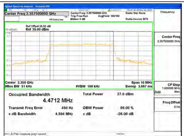
B40-2 / 5MHz / 16QAM/ High CH
