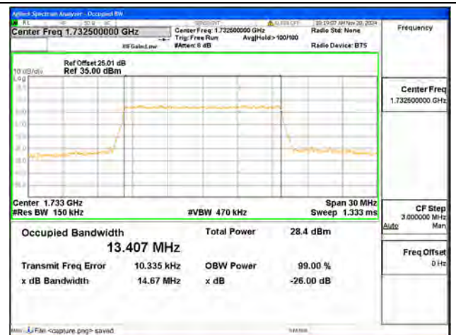
B4 / 15MHz / 64QAM/ Mid CH
