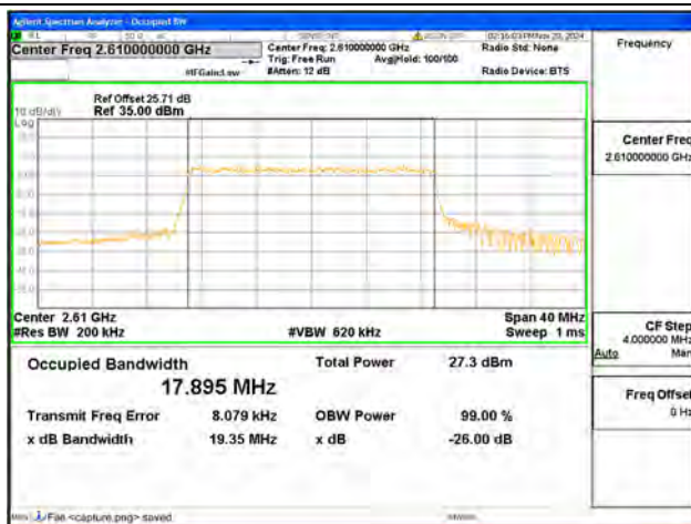
B38 / 20MHz / 16QAM/ High CH
