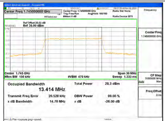
B66 / 15MHz / 64QAM/ Mid CH
