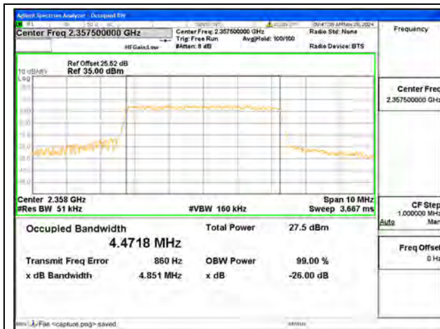
B40-2 / 5MHz / QPSK/ High CH
