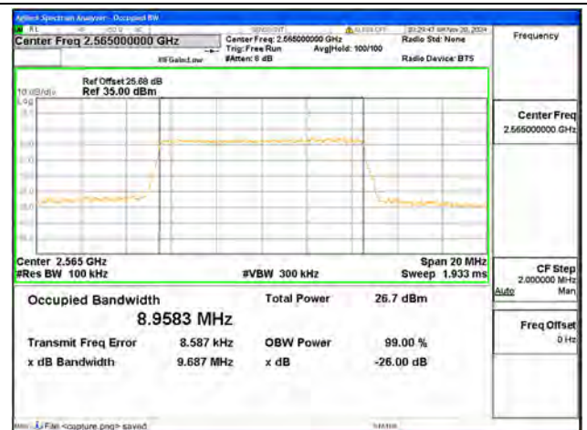
B7 / 10MHz / 64QAM/ High CH
