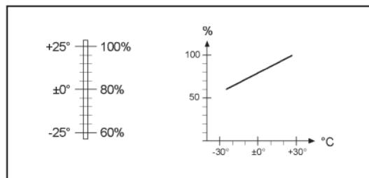
*Battery capacity at different temperatures.*
