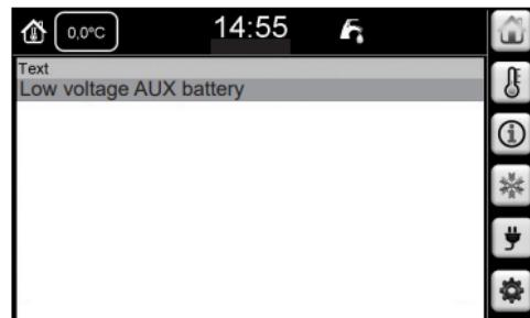
The electrical system resets automatically when the battery is fully charged. Fully charging the battery takes a number of hours.
