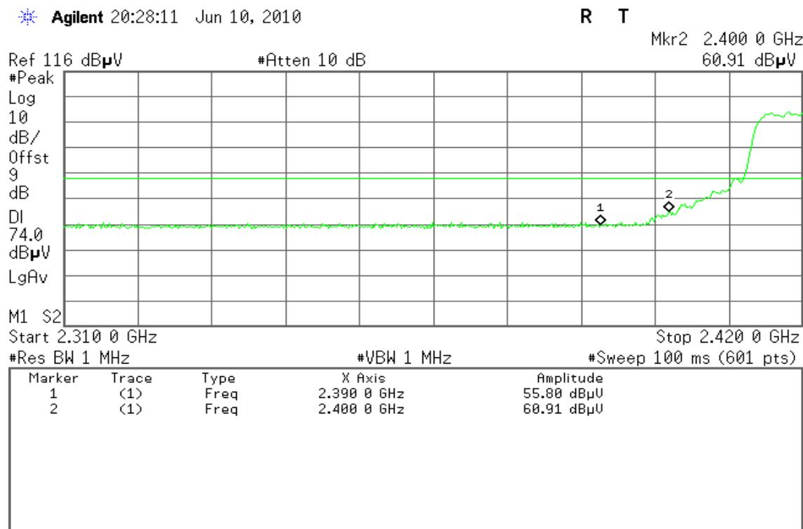
**Detector mode: Average****Polarity: Horizontal**
