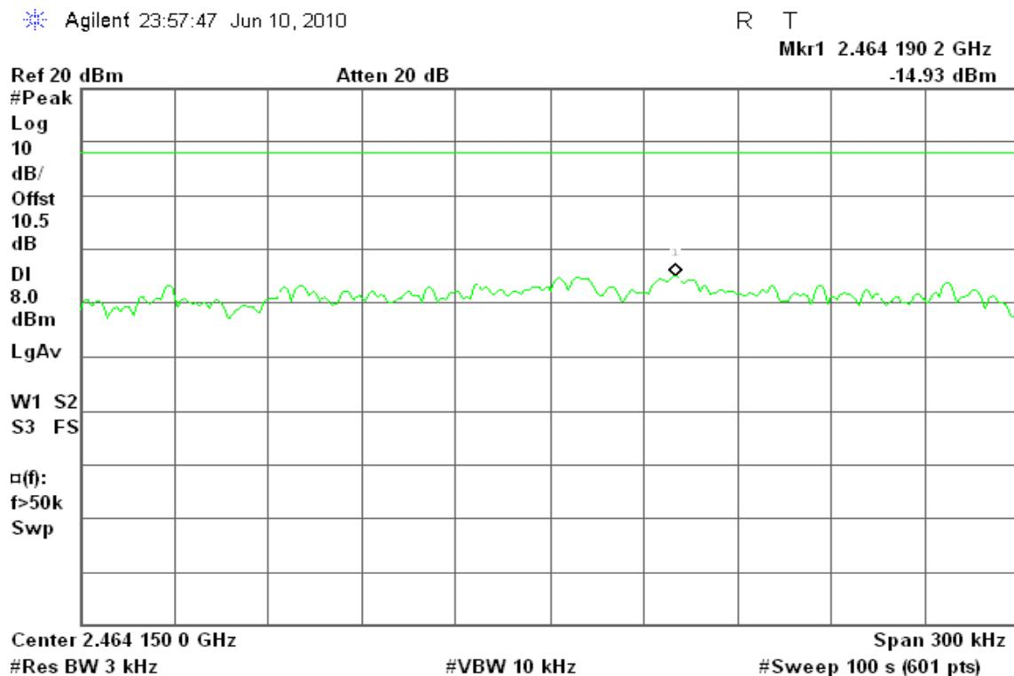
**draft 802.11n Standard-20 MHz Channel mode / Chain 1****PPSD (CH Low)**
