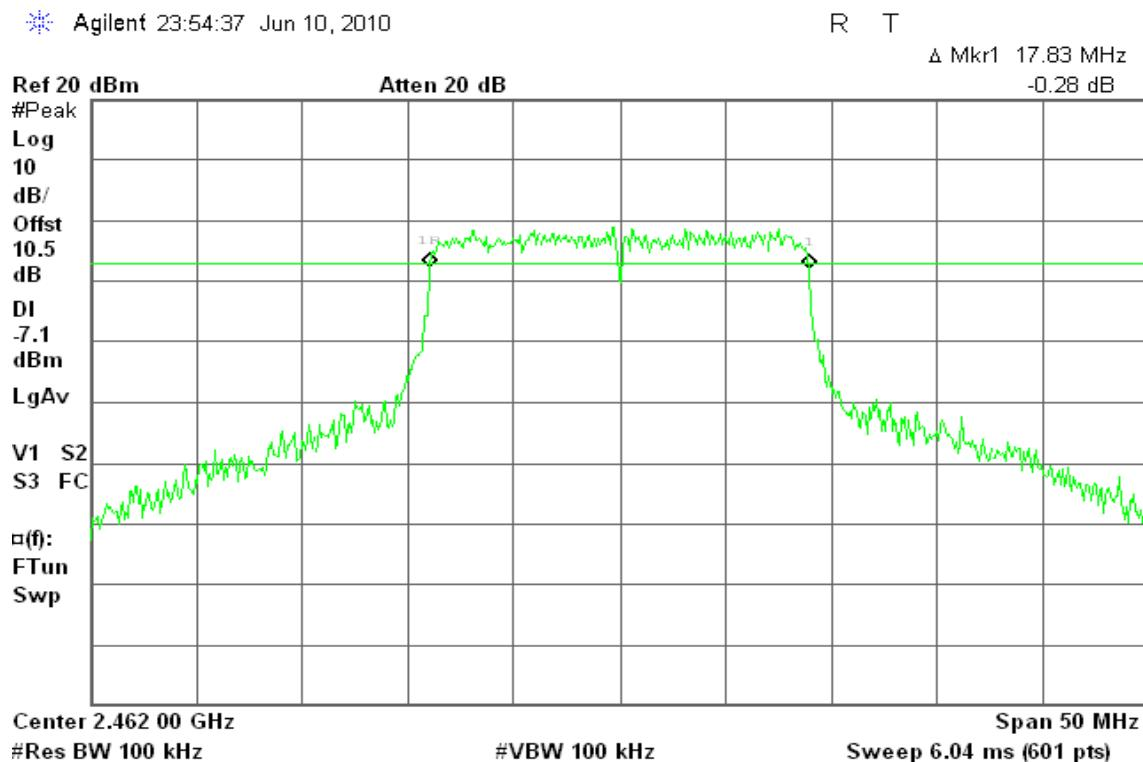
**draft 802.11n Standard-20 MHz Channel mode / Chain 1****6dB Bandwidth (CH Low)**
