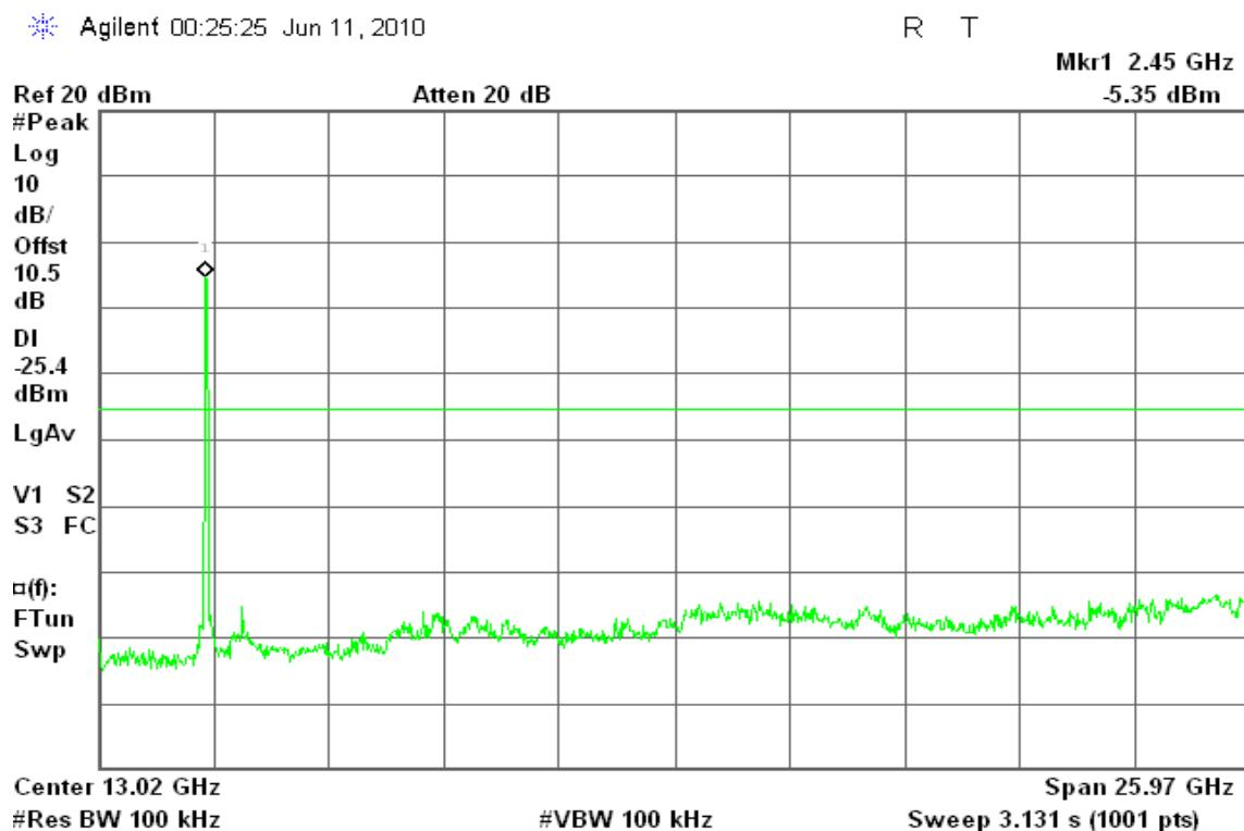
**draft 802.11n Wide-40 MHz Channel mode / Chain 1****CH Low**
