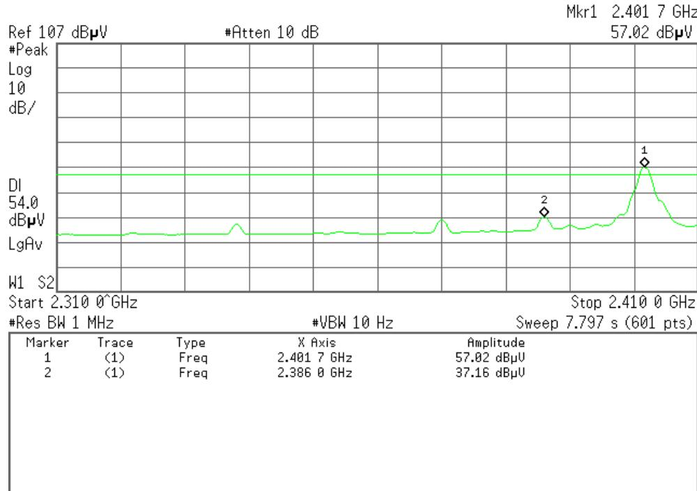
**Band Edges (CH-High)****Detector mode: Peak****Polarity: Vertical**
