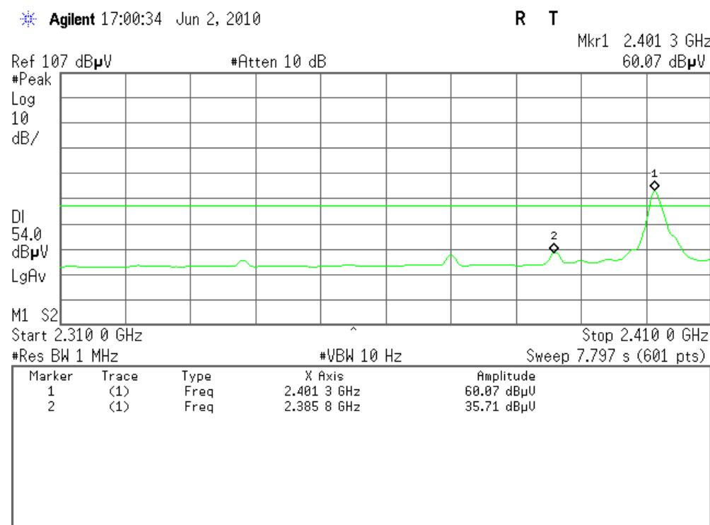
**Detector mode: Peak****Polarity: Horizontal**
