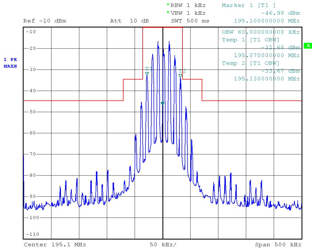
Emission Mask: input with 15 kHz AF, 50% modulation + 16dB.
