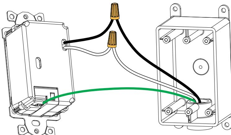
Field installed earthing conductor shall be equivalent or larger than the supply leads, 16 AWG minimum.
