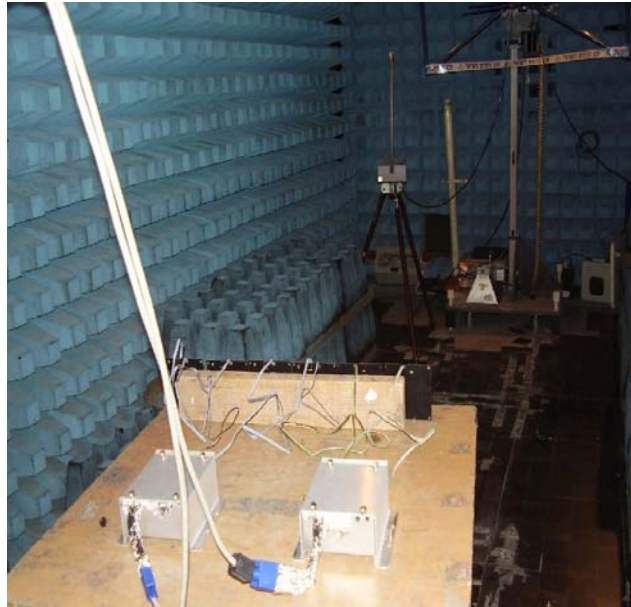
Photo 1. RE test in anechoic chamber.
