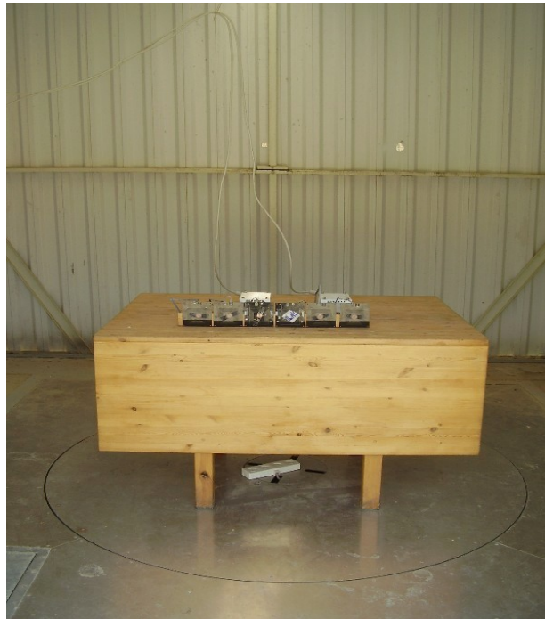
Photo 3. RE test setup on OATS.
