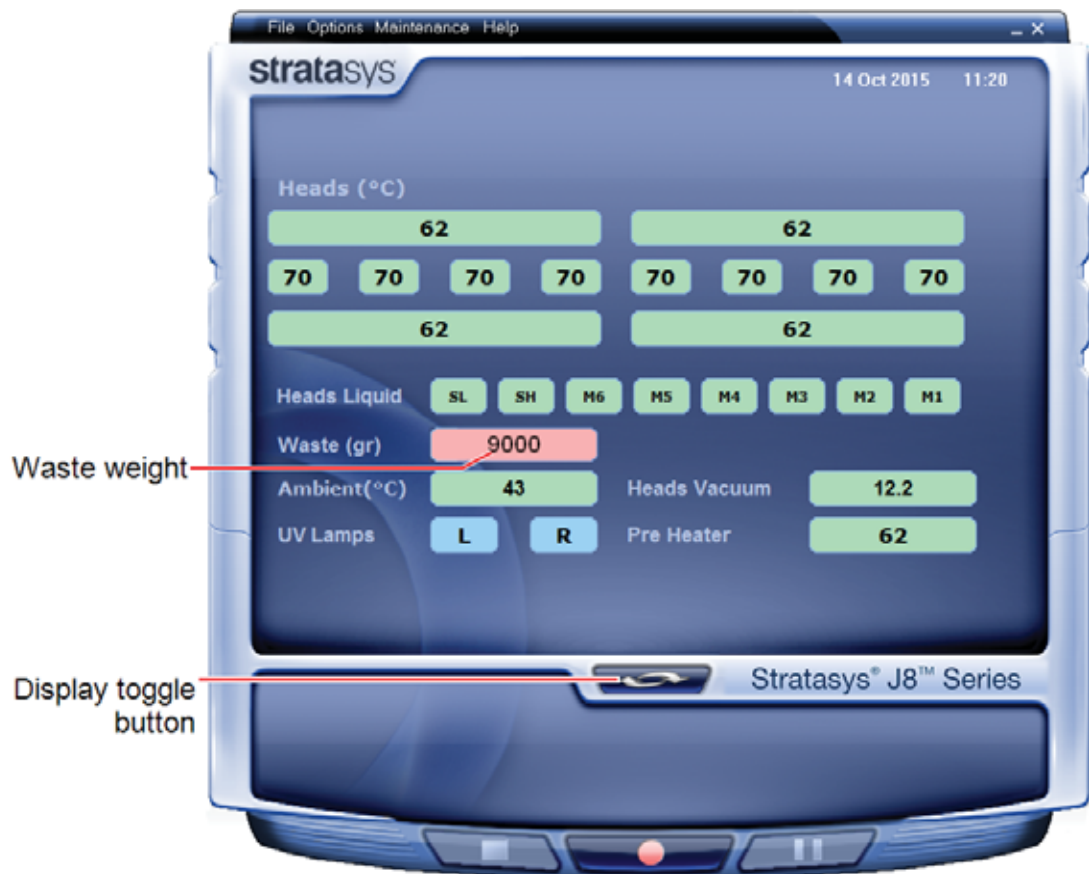
Figure 4-142 Printer interface, showing waste weight (red background indicates operator alert)
