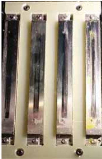
Figure 4-65 Print-head splash shield installed on the print block
