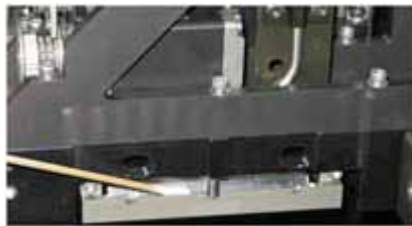
Figure 4-47 Cleaning the roller waste collector
