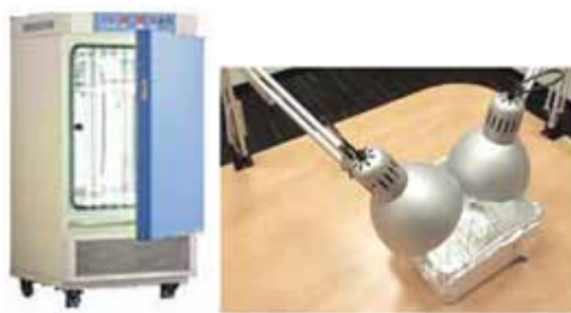
Figure 5-2 Left: Illumination chamber; Right: Desk lamps
