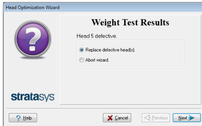
Figure 4-79 Defective print heads found
